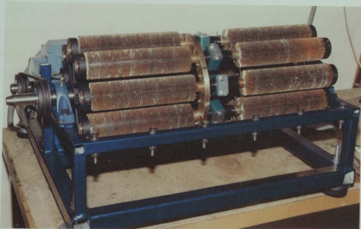
Photograph 6.8: 9-Pipe Wire Finned Rig
