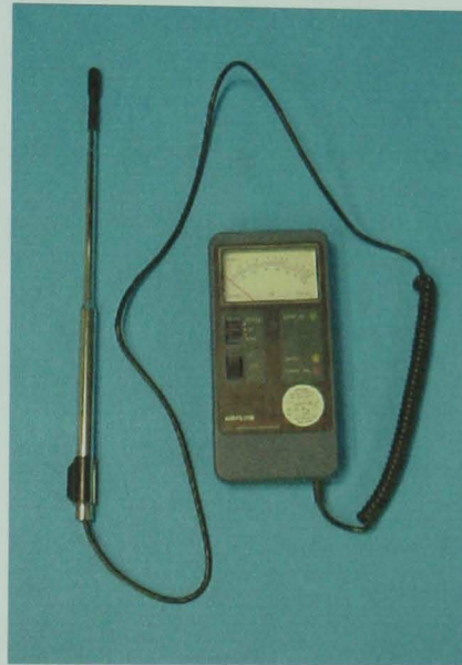
Photograph 7.4: Air velocity Probe (hot wire anemometer)
