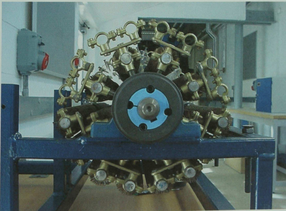
Photograph 6.14: 24-Pipe Rig: Pipe Clamps
