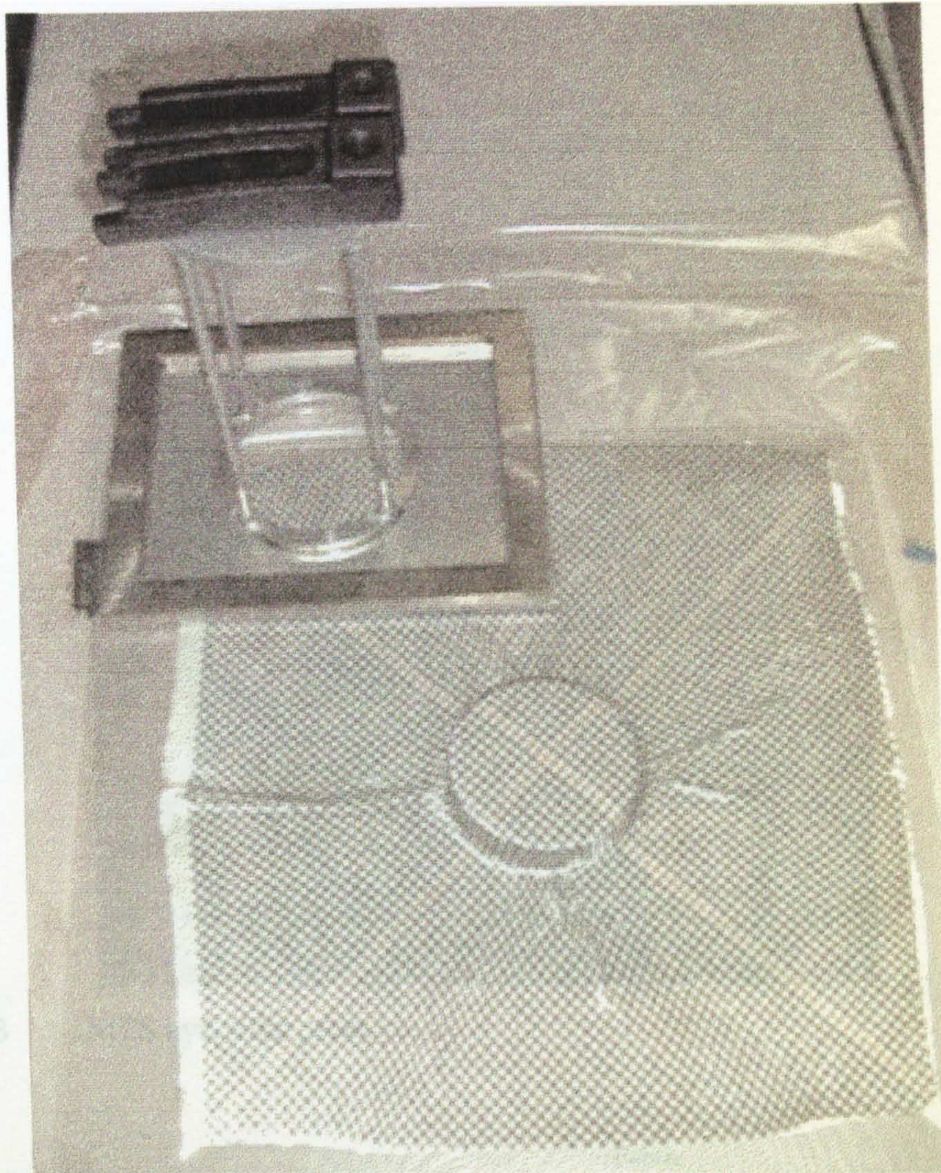
Figure 5.1 Vacuum assisted preforming equipment for disc geometry.
