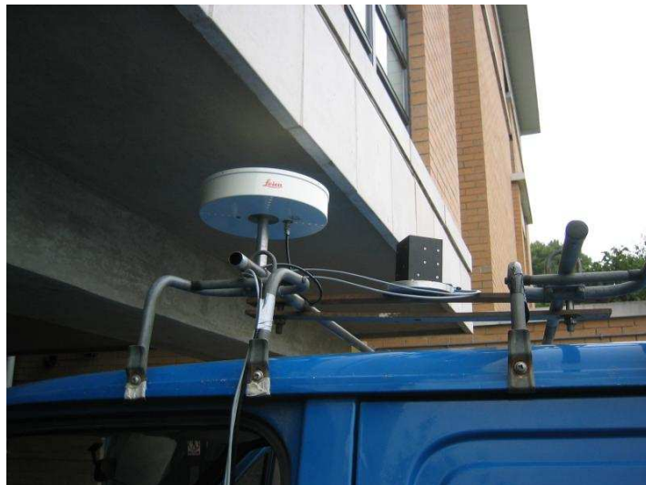
Figure 8.16: Crossbow AHRS-DMU-HDX and Leica choke ring GPS antenna mounted on roof of van
