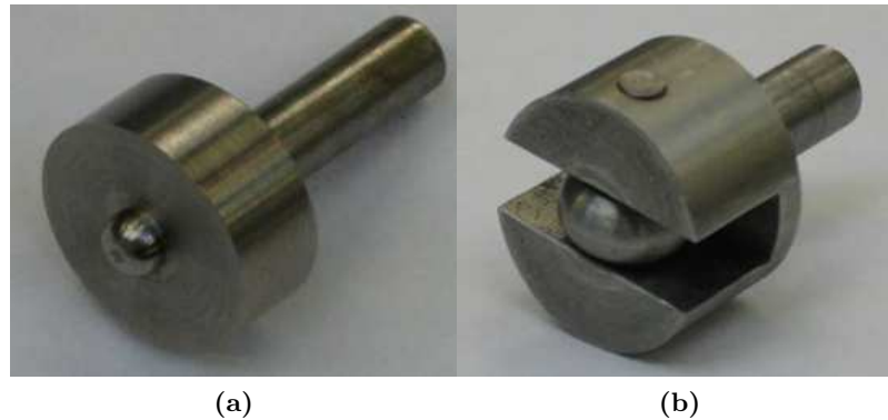
Figure 7.11: The two active element tips used for the fully active fixture. (a) A normal point-contact fixture tip that is used when the active elements maintain their position or change it in a discrete fashion. (b) A rolling point-contact tip enabling constant movement of the active elements with the need to disengage the workpiece surface.
