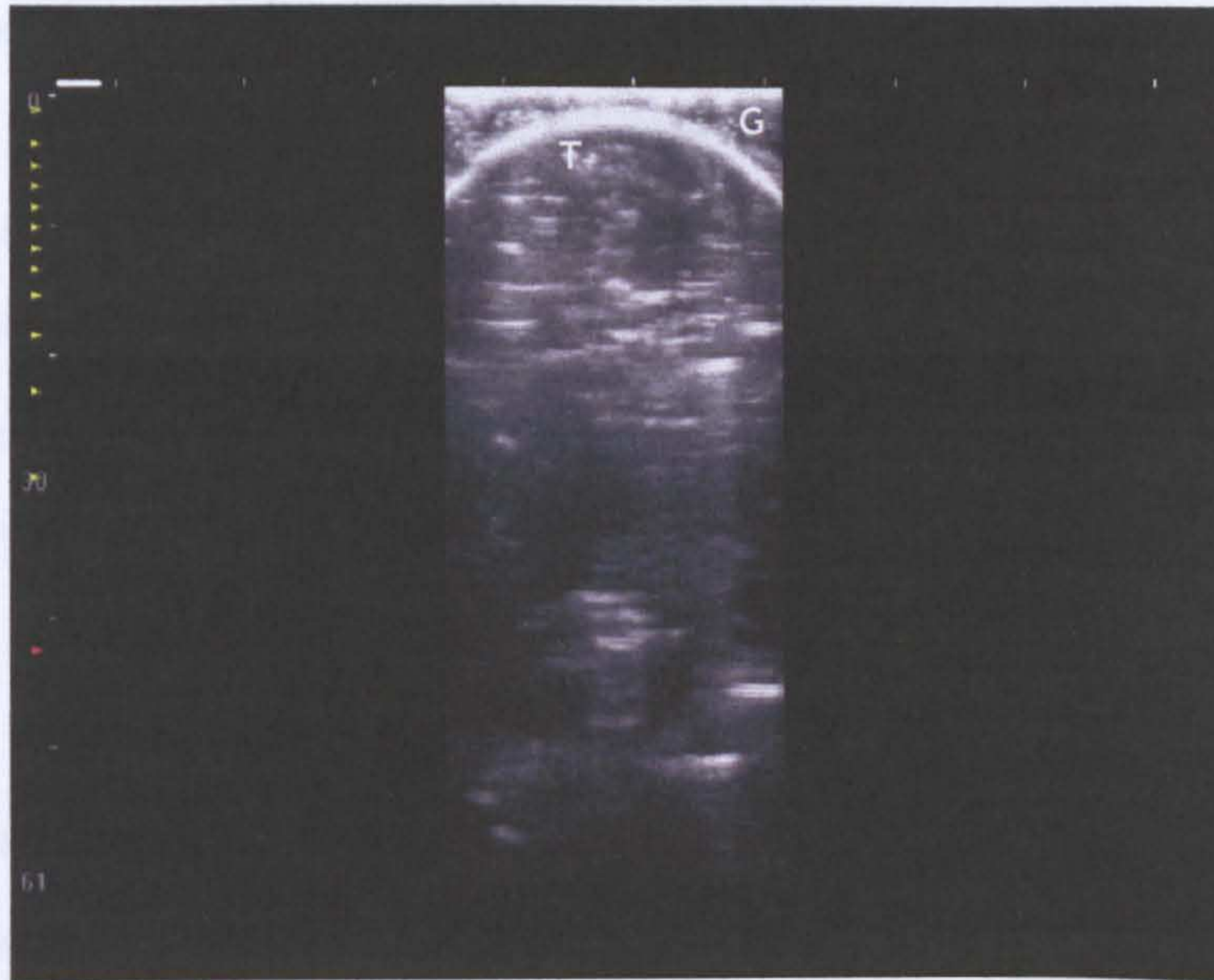
Figure 71: Ultrasound of spherical synthetic lesion Transverse scan (T = table tennis ball, G = gelatine)
