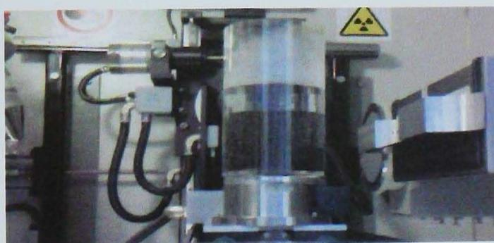
Figure 6.4 Specimen X ray scanning in water
