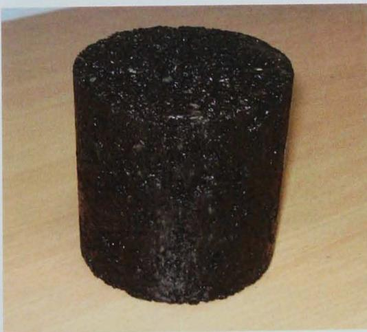
Figure 4.2 Specimen for monotonic compression test
