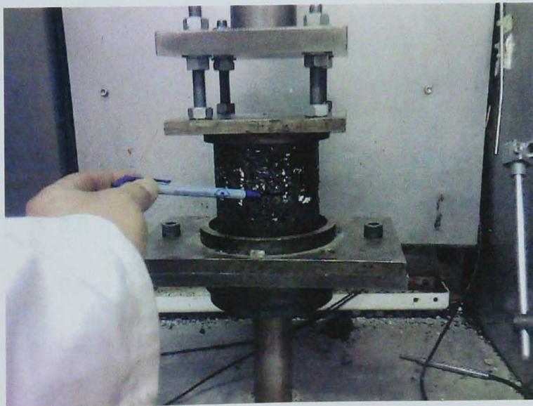
Figure 5.8 Specimen showing failure location after fatigue testing
