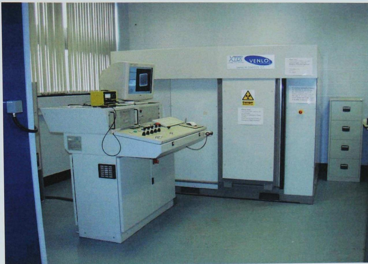
Figure 1. X-Ray CT System at NTEC, University of Nottingham
