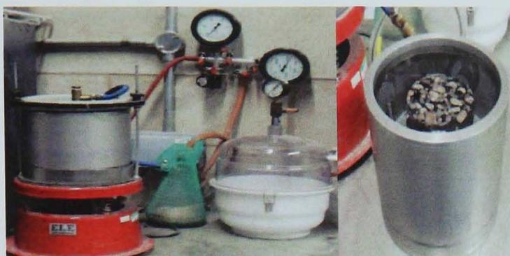
Figure 6.3 Laboratory setting for saturating the specimen
