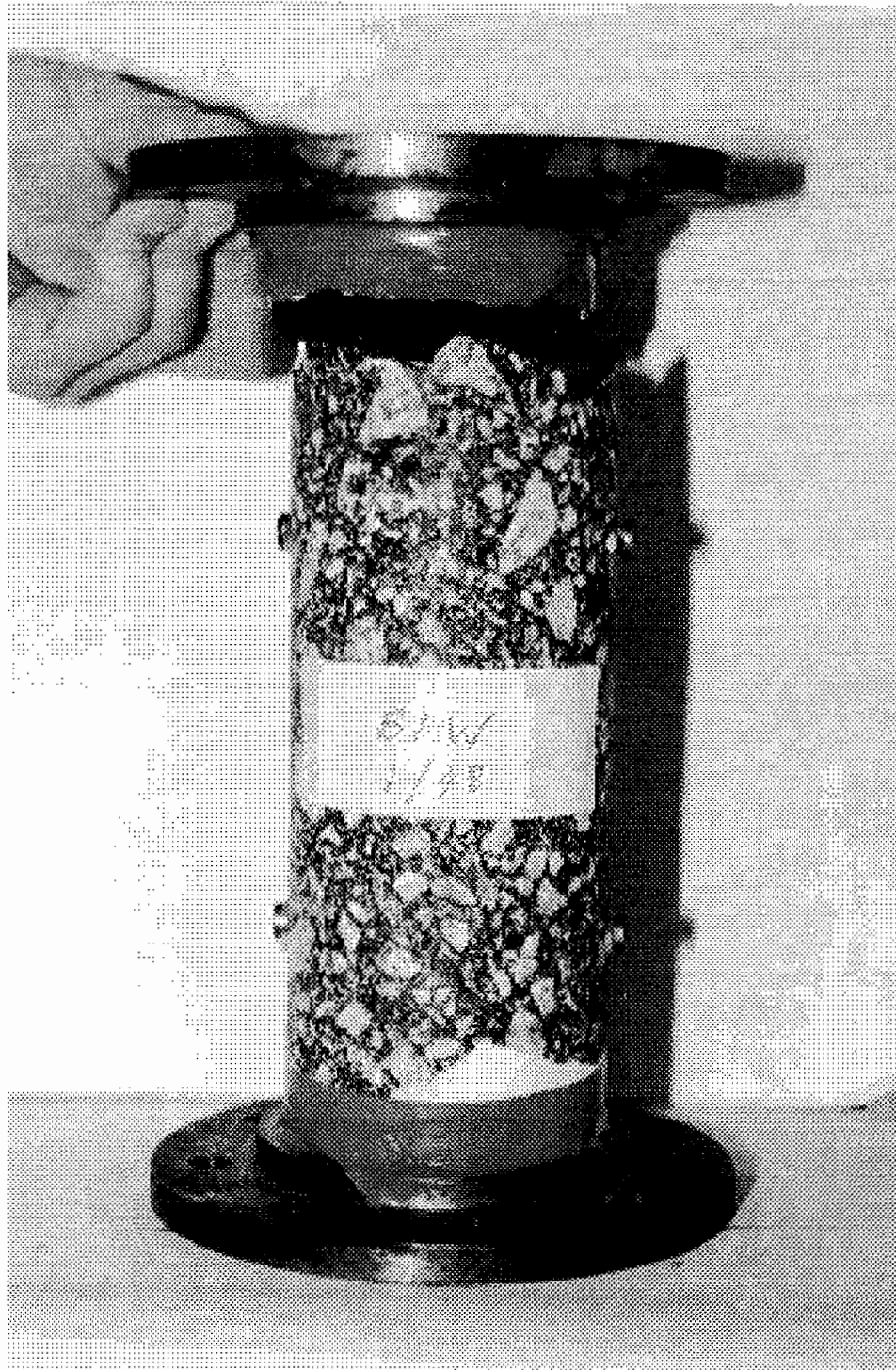
Figure 5.6 : Failed Specimen - Uniaxial Tension-Compression Fatigue Test
