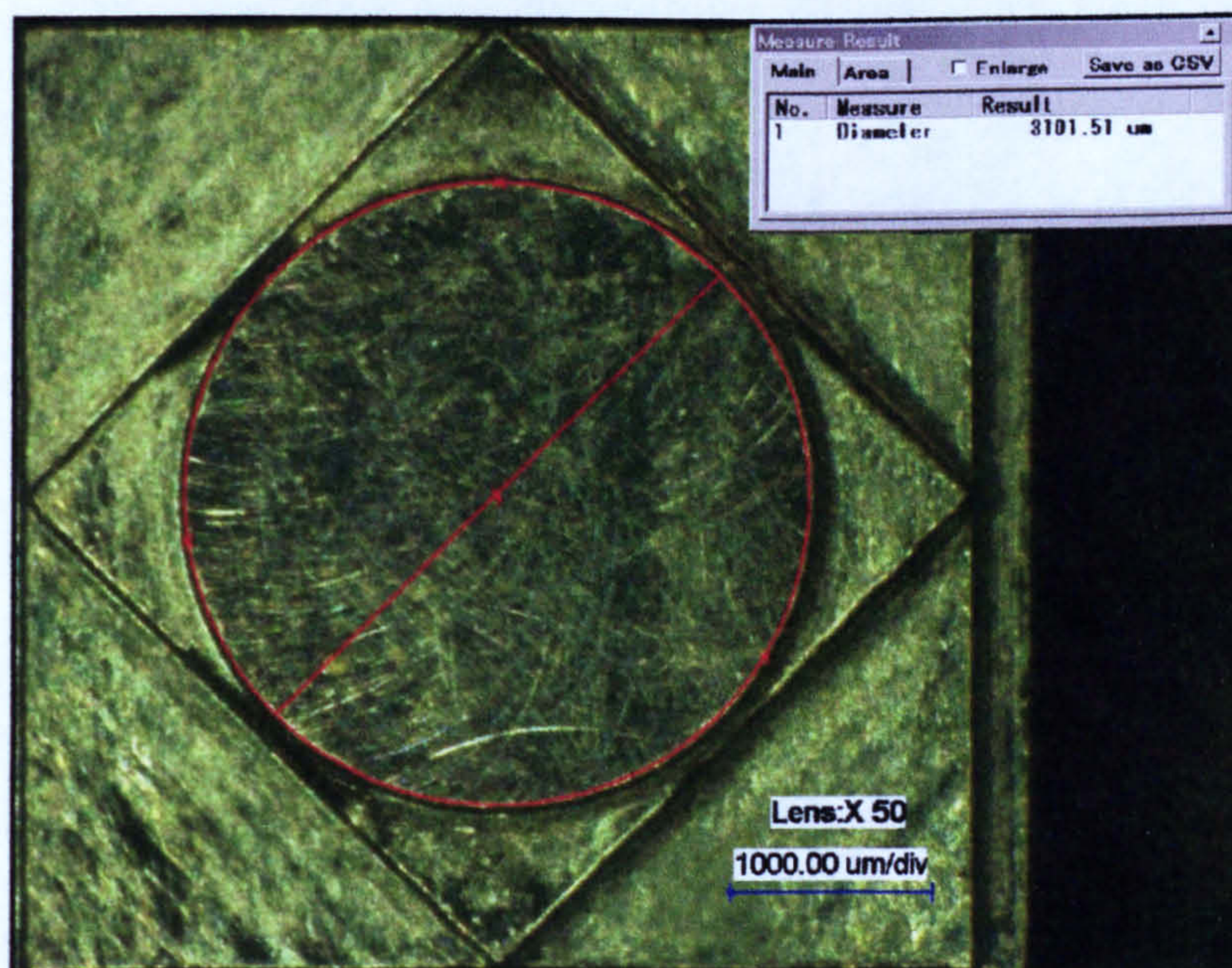
Figure 3.10 The example of on screen image of measuring the cylinder
