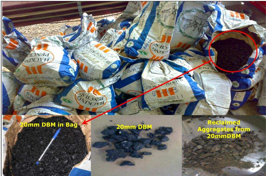
Figure 5.4: 20mm DBM (inset at the bottom right hand corner shows the appearance of reclaimed aggregates from the 20mm DBM)
