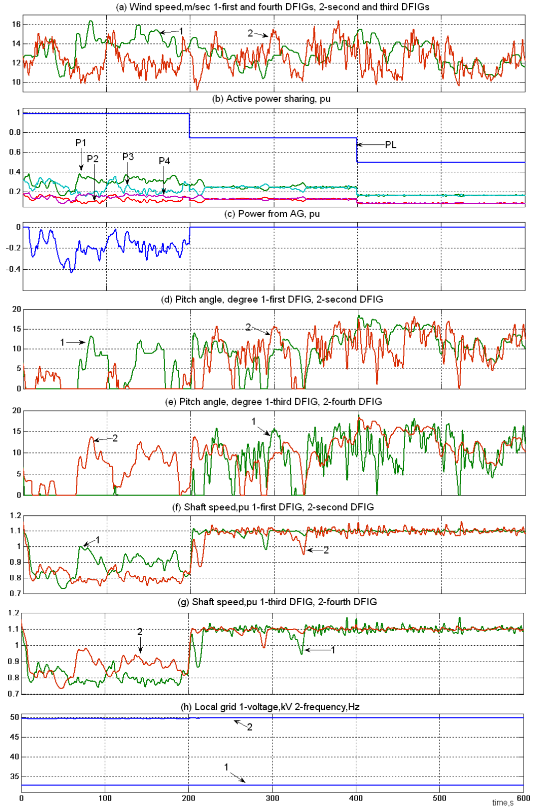
Figure 5.25. Power sharing of four simplified ISFO-controlled DFIGs the variable droop gain
