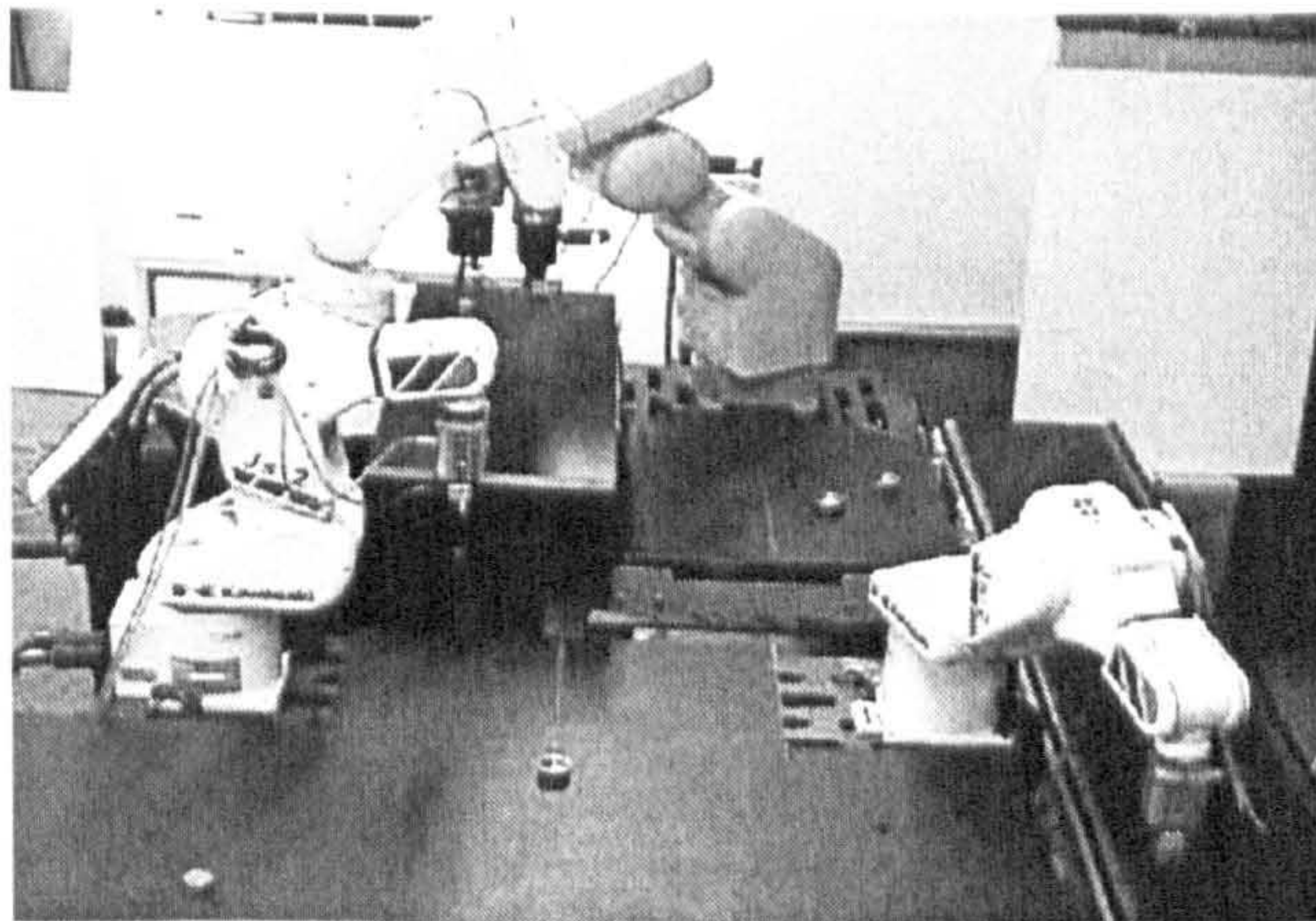
Figure 2.9 Holonic Assembly System Approach (Sugi, et al. [119])
