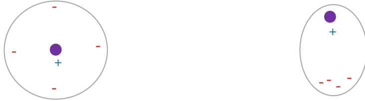
Figure 2.3 Electronic polarisation in a stable atom after nucleus is displaced with respect to surrounding electrons (Botsco and McMaster, 1986)
