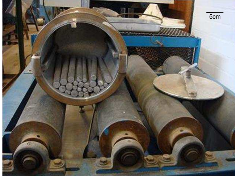
Figure 5.9 Laboratory rod mill used for grinding calibration tests and prior to liberation and flotation testing
