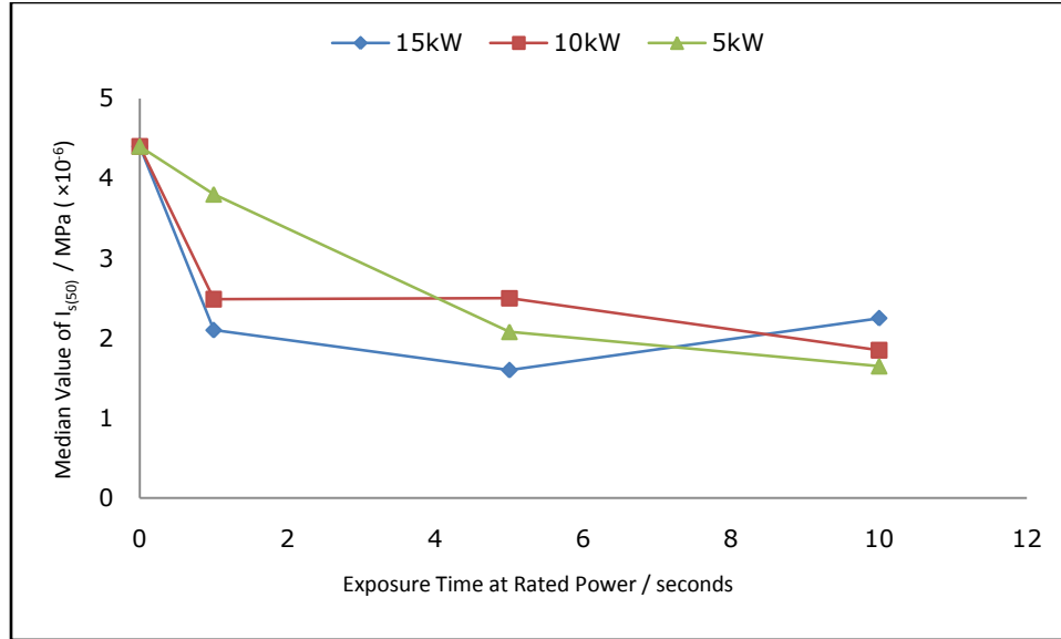
Figure 3.5 Variation of Point Load Index with microwave power and exposure time in multimode cavity (Kingman et al., 2004)
