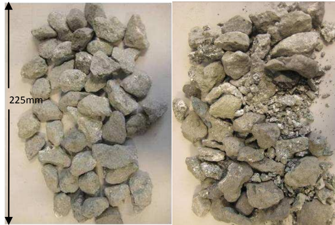
Figure 4.27 Kimberlite type II ore before and after microwave treatment
