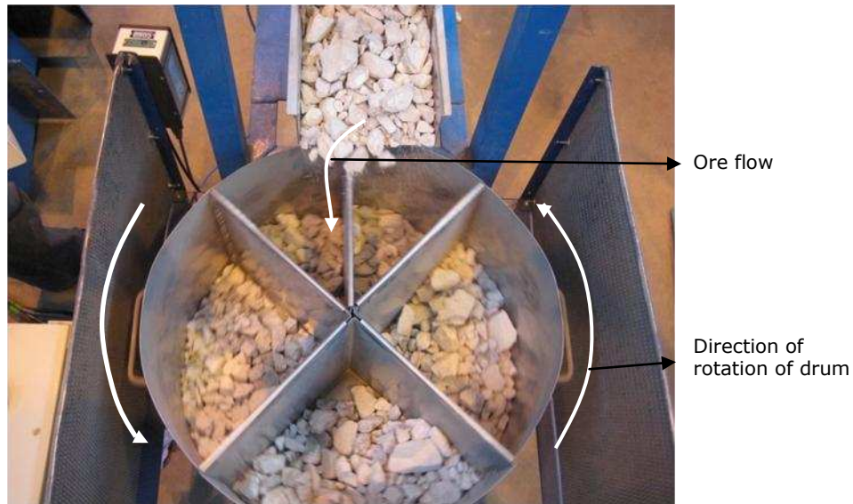
Figure 4.2 Rotary sample divider (RSD) used for ore sampling
