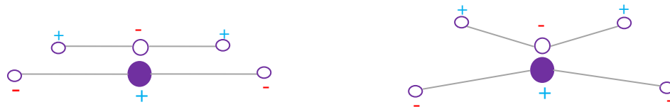
Figure 2.4 Atomic polarisation as result of nuclei displacement of different atoms (Botsco and McMaster, 1986)
