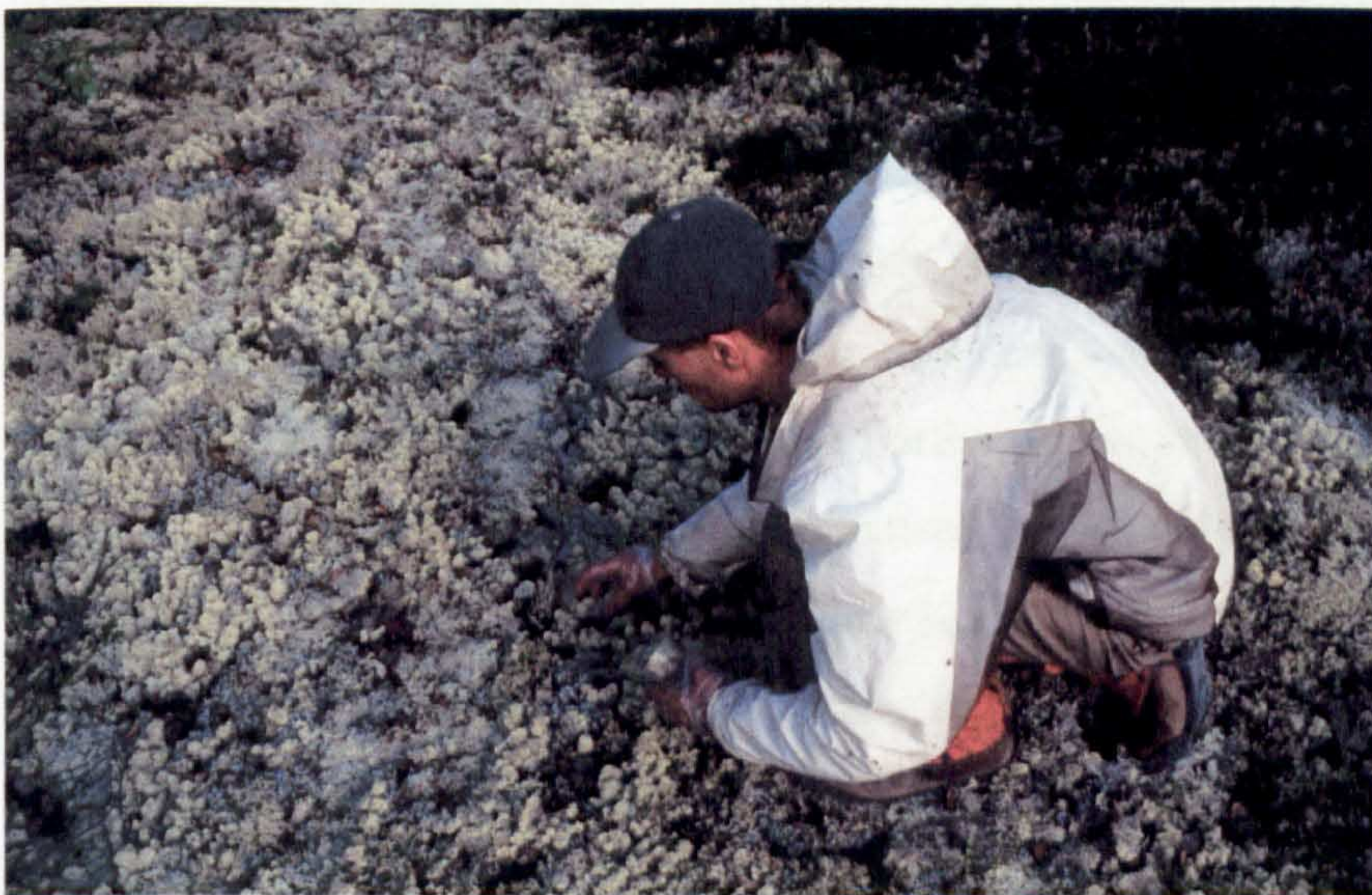
Figure 2.4. Lichen sampling using LDPE containers and powder-free LDPE gloves to minimise contamination. (Photo: P Kuhry).
