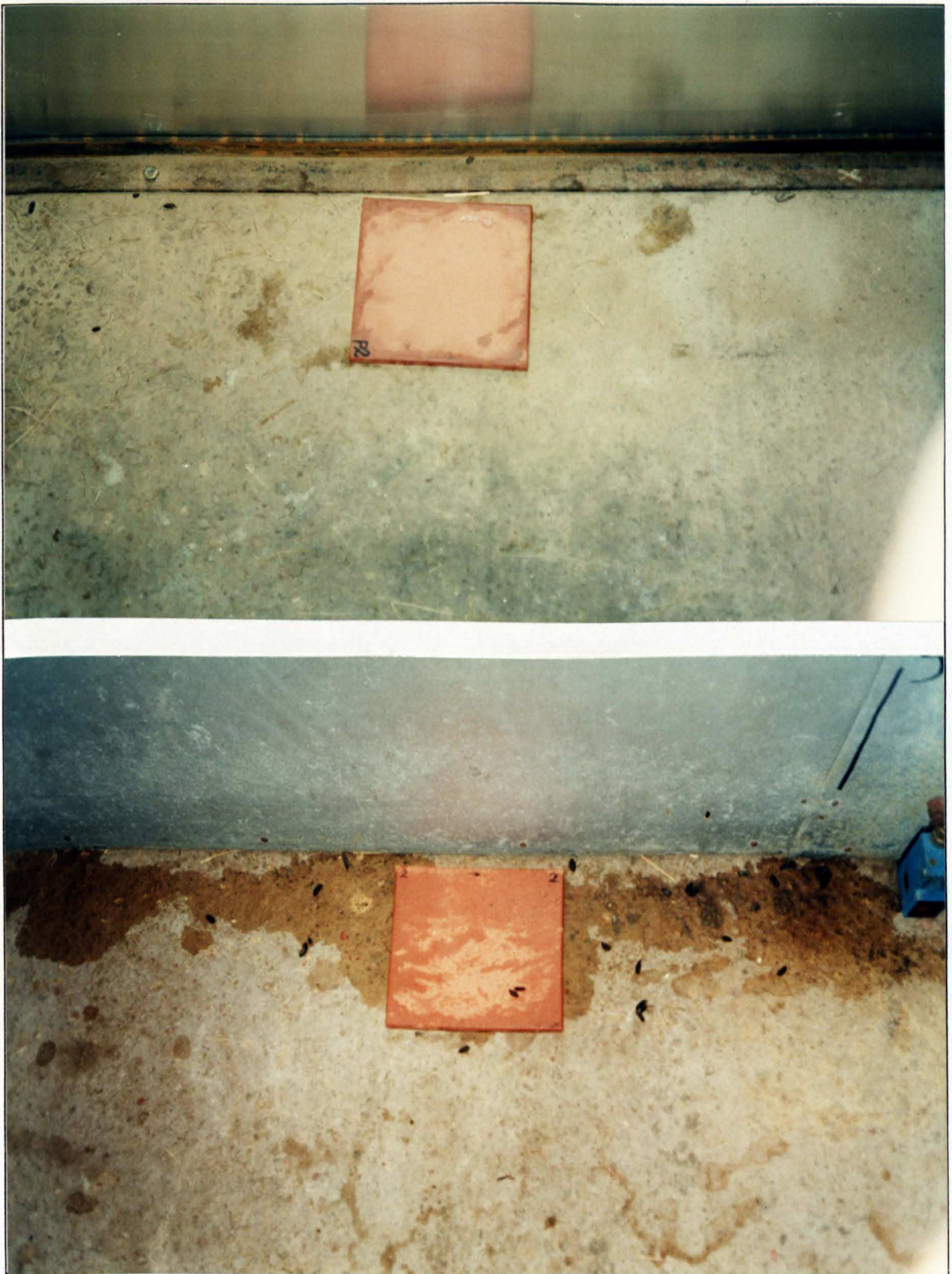
Plate 4.2. Extent of marks on a previously clean tile after it had been marked overnight in a pen (upper photograph, first part of the test), and after a similarly marked tile had then been transferred to a neighbouring pen for a second night (bottom photograph, second part of the test). The dark areas indicate urine marks. The increase in surface covered by marks was remarkable, especially when the stimuli were marks from neighbour rats (bottom photograph). In this case it was common to find faeces around the tile (faecal marking). Both are representative of each stage of the test.
