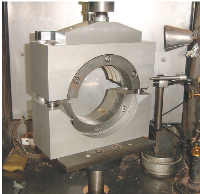
Figure 2.38 – Photograph of the Leutner shear testing device (From Choi et al. , 2005)
