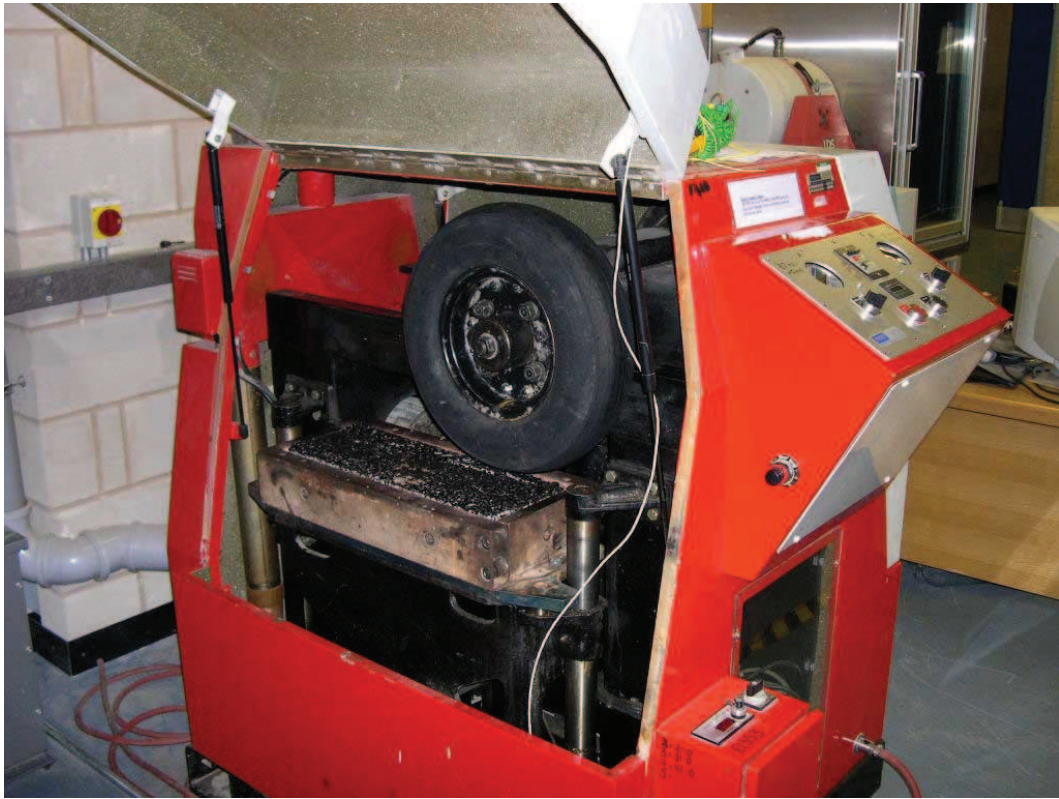
Figure 5.12 – Trafficking setup for FWT
