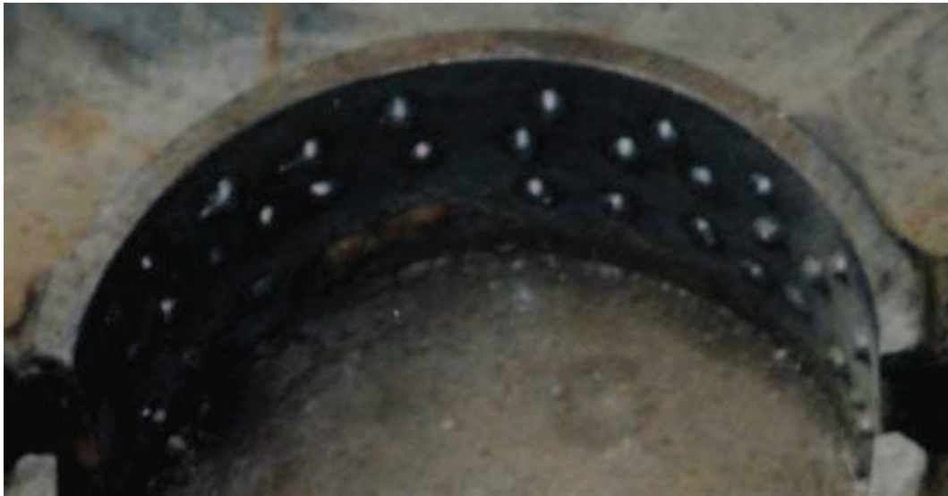
Figure 4.8 – Small welding patches applied into the inner surface of the clamping unit
