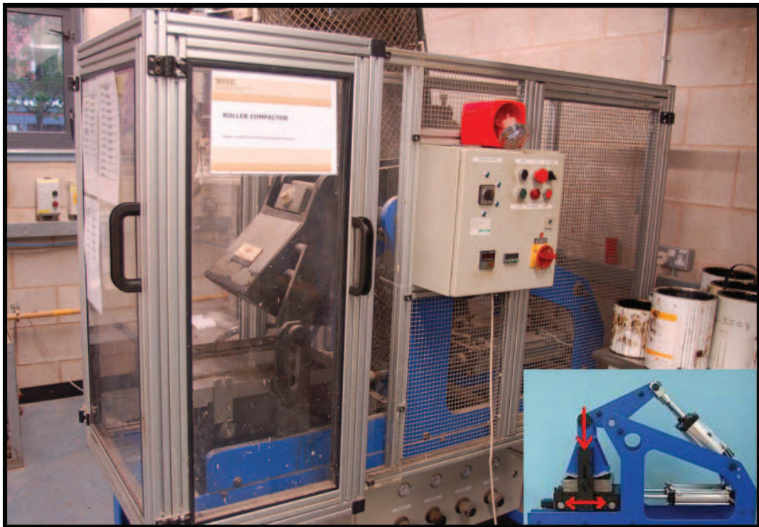
Figure 3.2 - Photograph of the slab roller compactor
