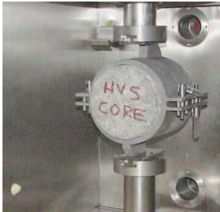
Figure 2.44 – Shear testing device developed by Sholar et al. [2004]
