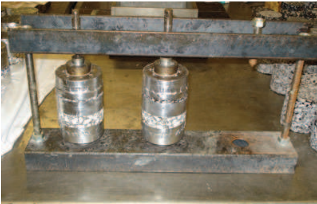
Figure 4.5 – Jig for gluing the loading platens to the torque specimens
