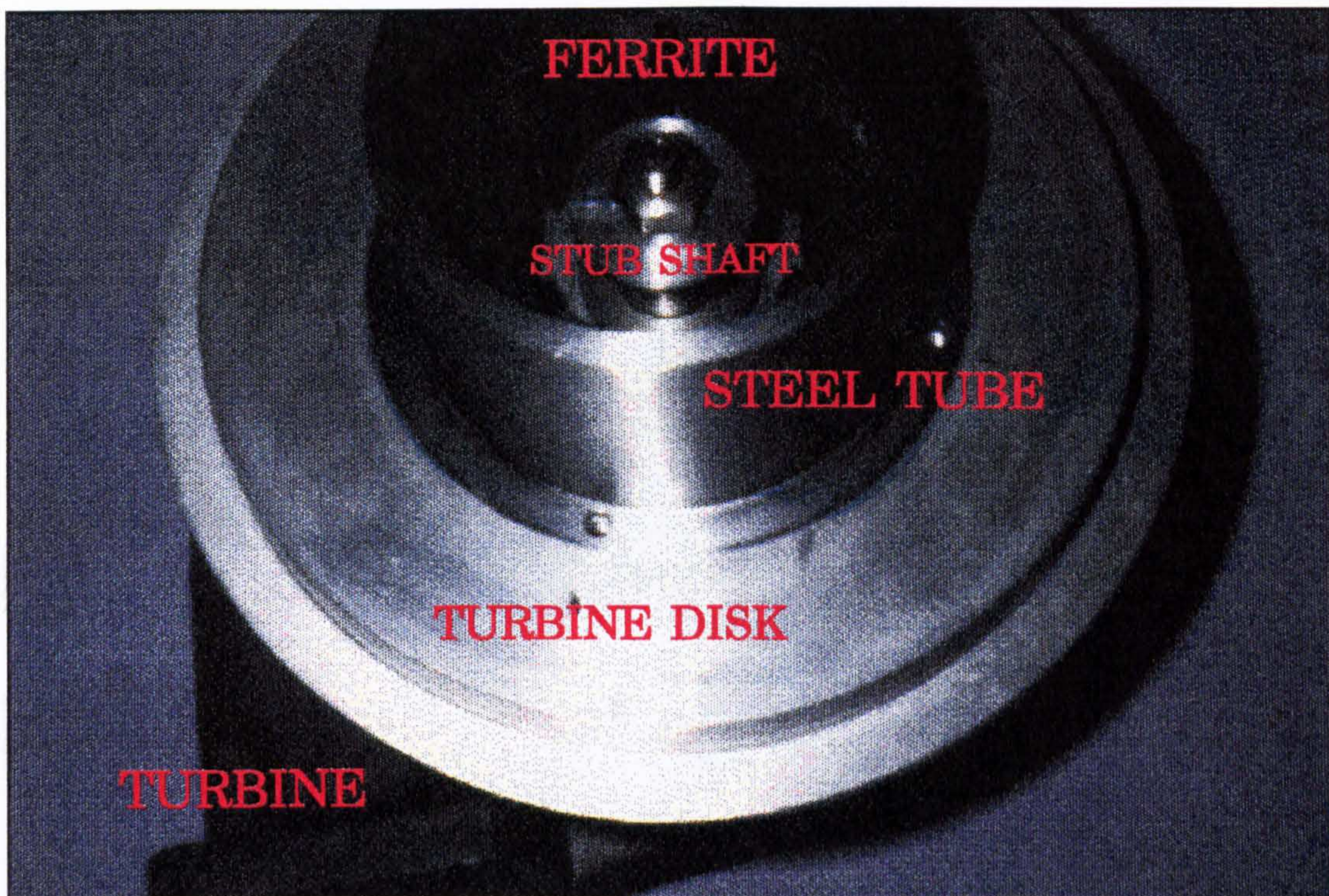
Figure 4.13: Photo showing the stator core inside the steel tube and its assembly to the air turbine.
