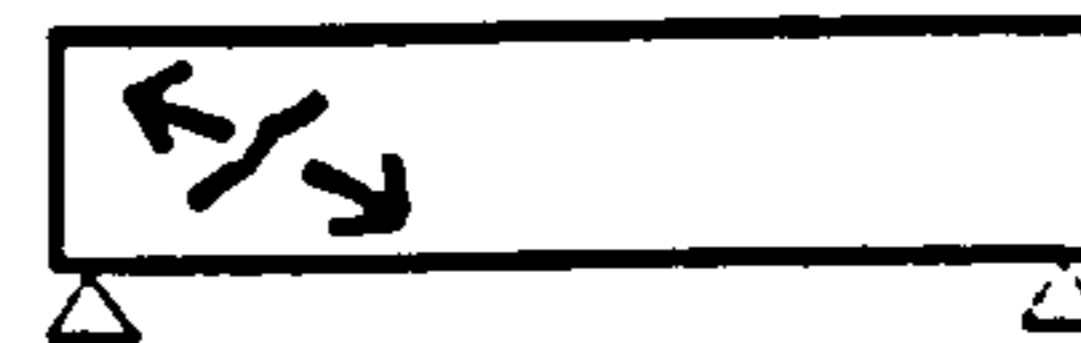
d) Web shear tension failure of concrete
