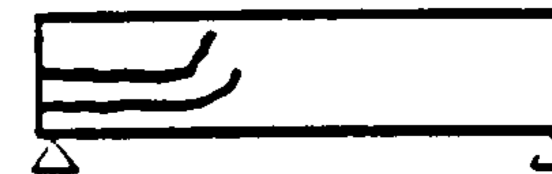
e) Longitudinal web shear cracking of concrete or longitudinal shear cracking of concrete at strand level
