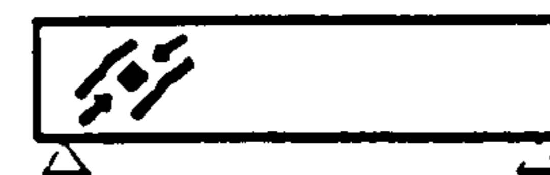
f) Web shear compression failure of concrete
