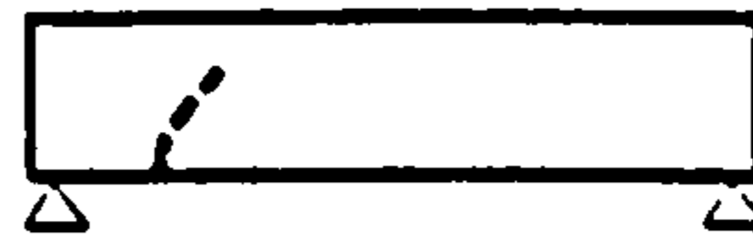
a) Flexural shear cracking of concrete
