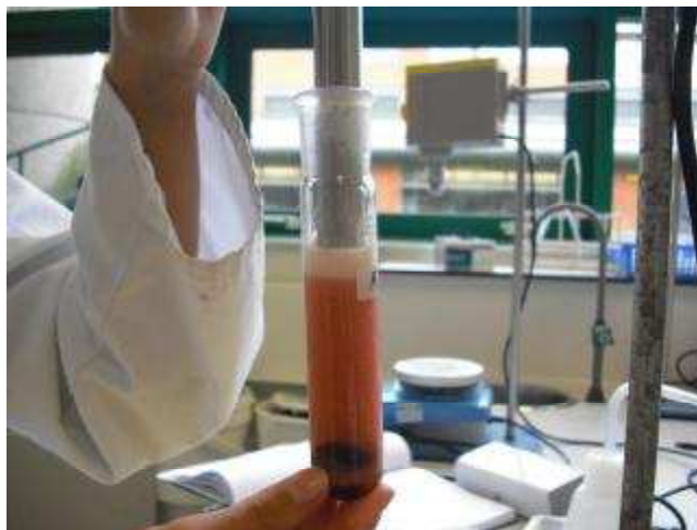
Figure 3.3: Homogenisation of the cherry tissue in distilled water with the presence of \text{CaCl}_2
