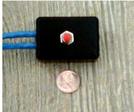
Figure 7.6: A lag switch for cheating in games
