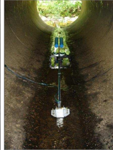
Figure 6.1 (a) Turbidity monitoring equipment, deployed in a culvert at (b) Sheepfold on the Nant Pen-y-cwm and (c) beneath Hrrhos Bridge on the Nant Melin-y-grûg.
