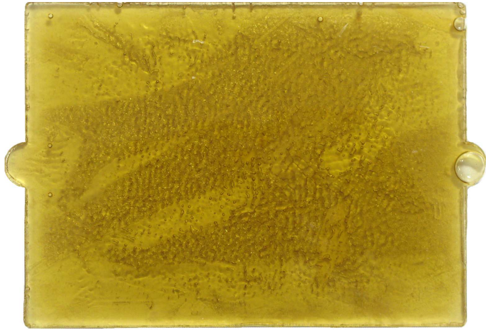
Figure 2-16. Casting of 100 PHR (parts per hundred resin) bisphenol A/F with 10 PHR photoinitiator UVI-6992. The dark yellow colour is due to the high photoinitiator compositional ratio. The specimen was cured in 20 mins using the flood lamp ( 0.1 \text{ W/cm}^2 ).
