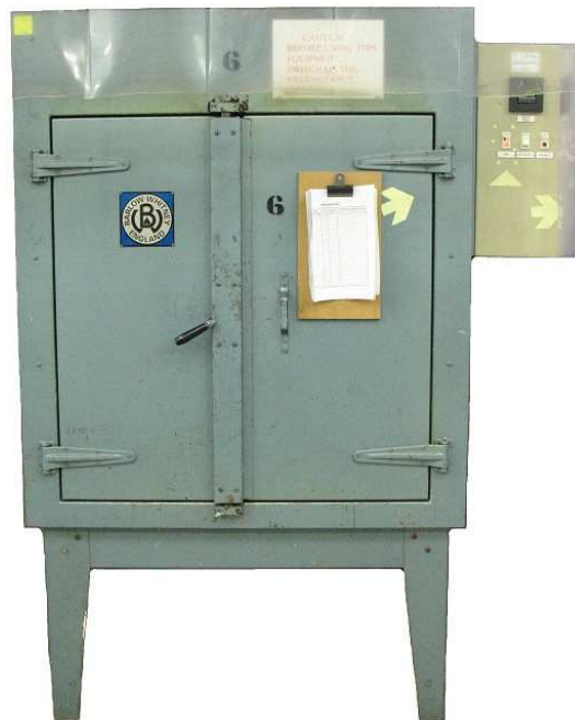
Figure C-5. Barlow Whitney oven used for heat treatment of the fibre samples wound on the aluminum tool (Figure 5-1 of Chapter 5).
