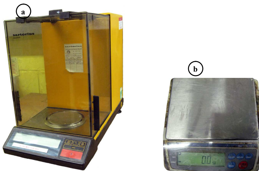
Figure C-1. Digital Weighing scale: (a) Sartorius HR60, (b) AND EK-1200i.
