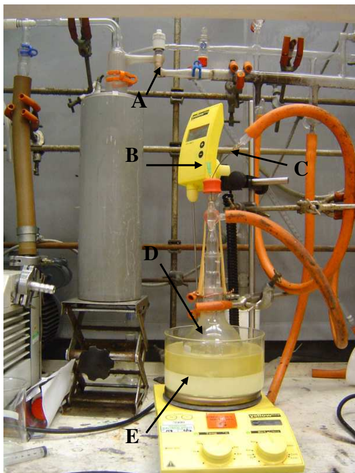
Figure 2.1: Photograph showing the set-up for synthesis of the triblock – PLGA-PEG-PLGA. A – Schlenk line; B – Injector used for the delivery of N_2 or argon gas into reaction chamber; C – Needle for pressure and gas outlet; D – round bottom flask; and E – liquid paraffin used for uniform heating of round bottom flask.
