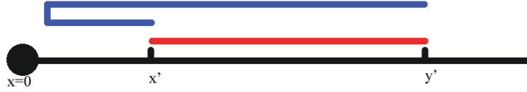
Figure 3.2: The two trips that connect two points x' and y' on a semi-infinite cable 0 \leq x < \infty . The red line represents the trip with length |x' - y'| and the blue trip has length x' + y'
