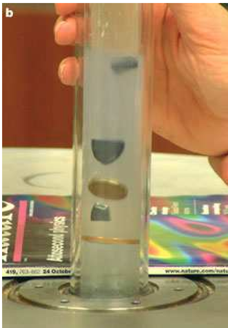
Figure A.2: Various objects were levitated above the bore of the 17T superconducting magnet in paramagnetic liquid oxygen. Figure taken from Catherall et al. [97].
