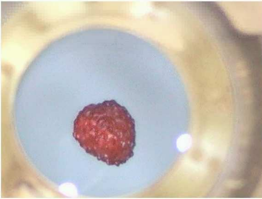
Figure A.1: A strawberry levitating. The strawberry is diamagnetic due to its high water content.
