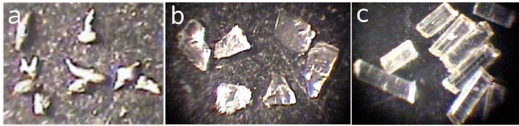
Figure 6.1: A photograph taken through a microscope, showing a bismuth grains, b non-spherical crushed glass, and c polymethyl-methacrylate (PMMA) rods formed from optic fibres cut into short lengths
