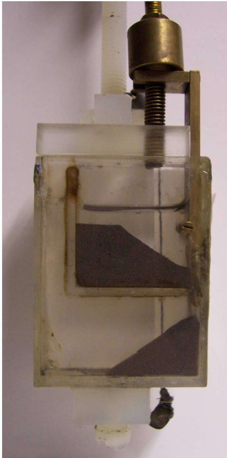
Figure 5.4: The draining aperture was closed with a wedge, which could be raised and lowered using a screw thread.
