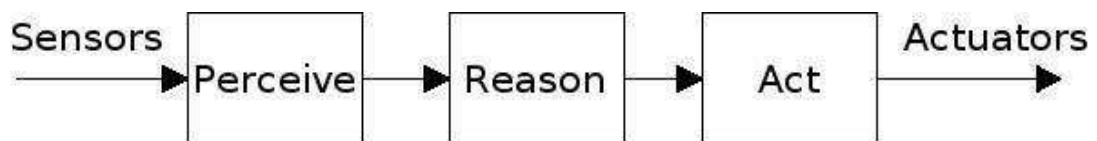
Figure 2.14: Robots collect information about the environment/task, decide what to do, then perform the necessary motor commands.
