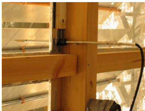
Figure 4.15 Air velocity transducer position inside the cavity, next to the inner skin.
