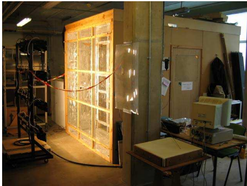
Figure 4.1 Experimental Facility: Box-Double Skin Facade Chamber at the School of the Built Environment of Nottingham University.
