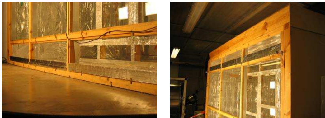
Figure 5.10 Inlets and outlets sizes adjusted with reflective panels on the external skin.
