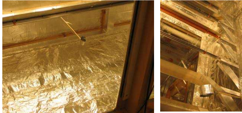
Figure 4.12 Shielded K-type thermo-couples inside the cavity.
