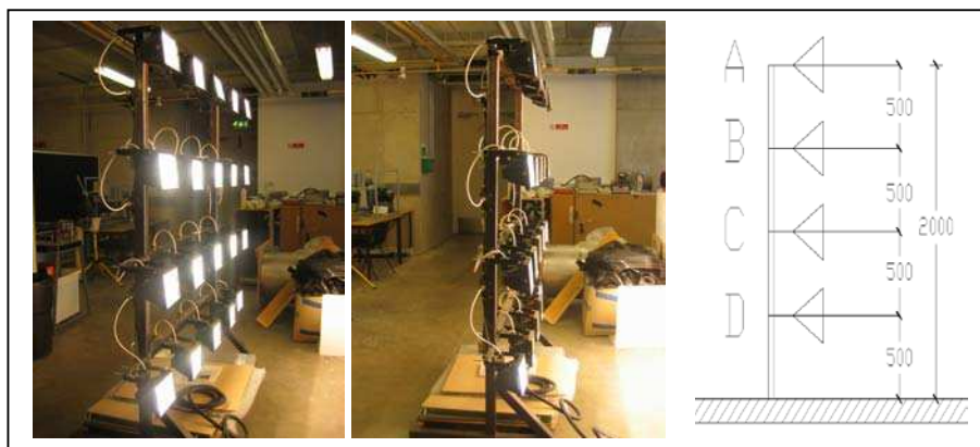
Figure 4.7 Solar simulator of the experimental facility.
