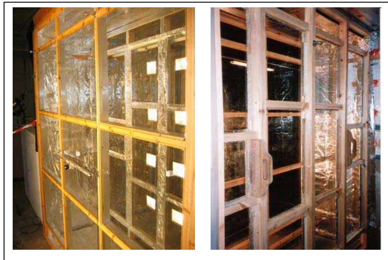
Figure 5.69 External and internal views of the DSF cavity adjusted to 800mm depth.
