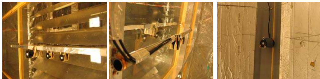
Figure 4.13 Radiation sensors located on the external, internal skins and back wall of the experimental chamber.
