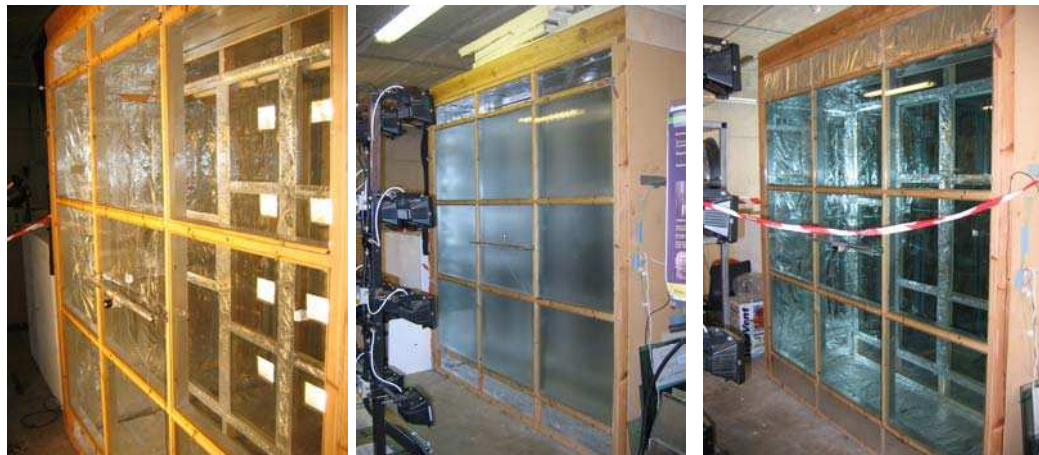
Figure 4.31 Clear, Textured and Green tinted glasses used in the experimental chamber.
