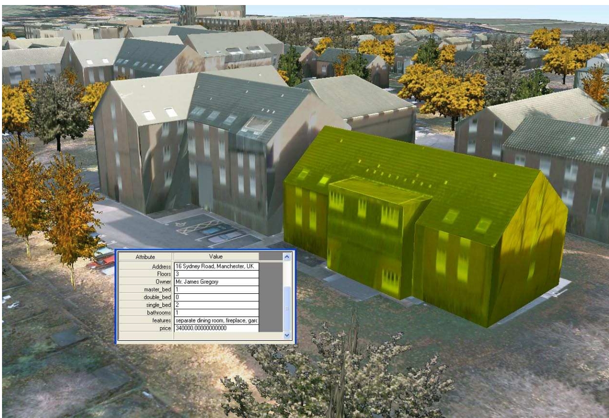
Figure 16 3D building models in Manchester area linked to a relational database in VirtualGIS™.
