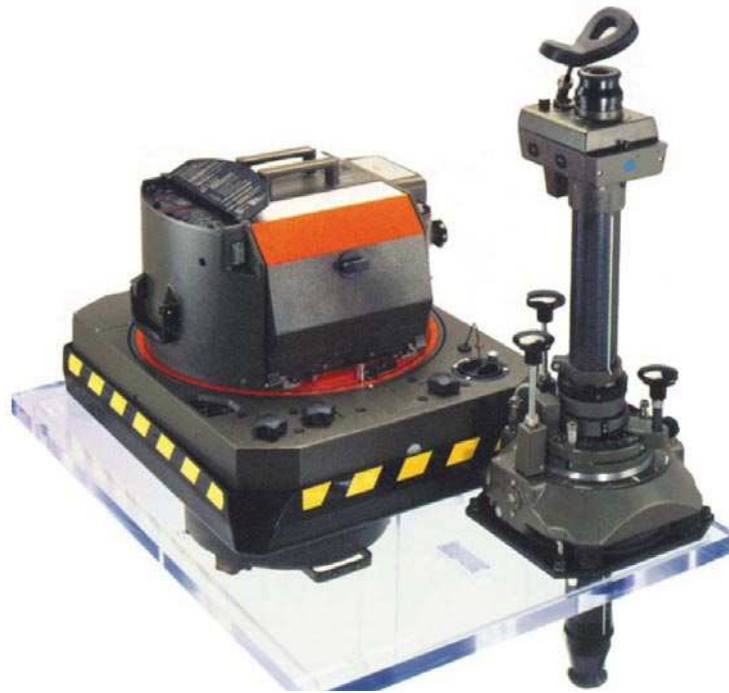
Figure 47. The Leica RC-30 aerial frame camera with navigation sight (adapted from Leica RC30 brochure, 2007, Copyrights reserved by Hexagon Corp.)
