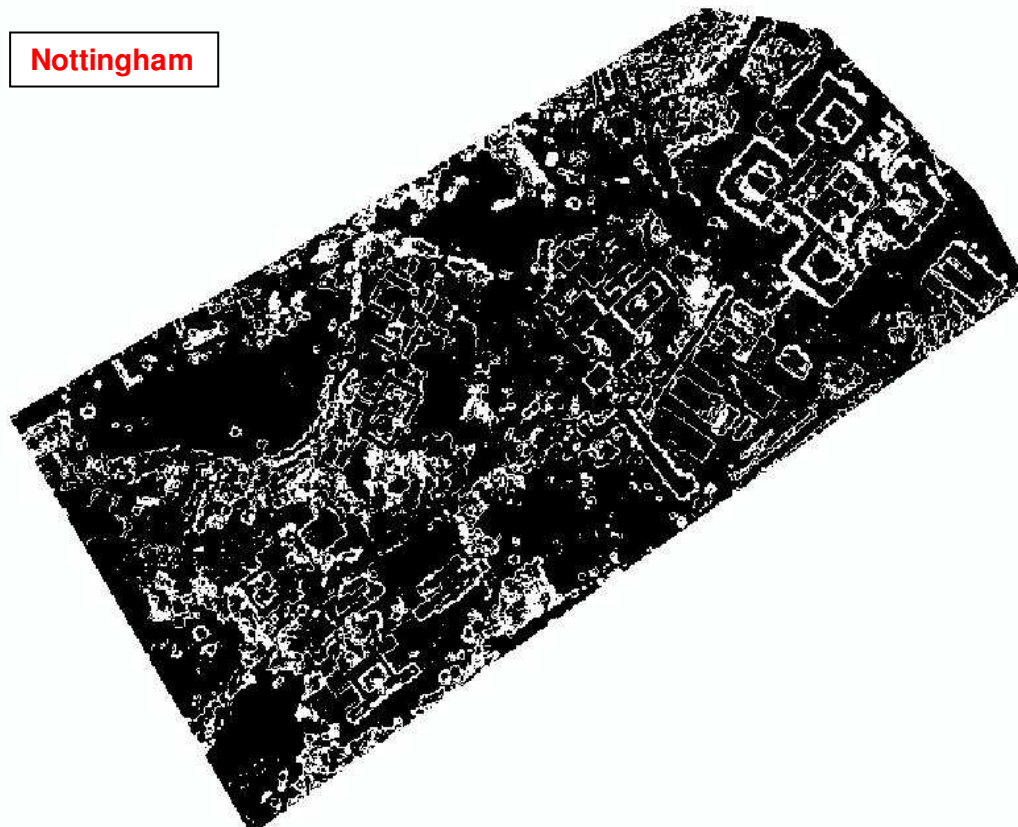
Figure 122 The resultant foreground and background object class from the implementation of the region growing segmentation workflow in second and third study areas 214
