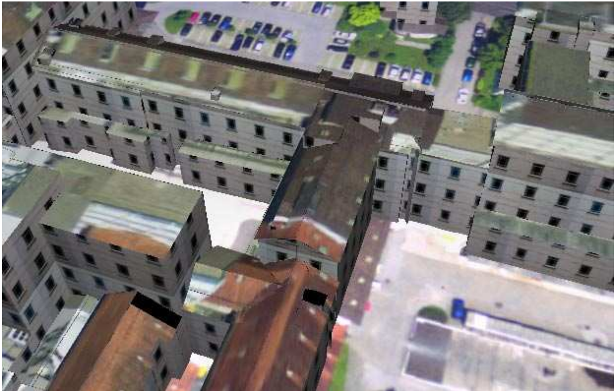
Figure 171 Detailed perspective view of the textured building models, superimposed on the orthorectified true color composite which was draped over a DSM
