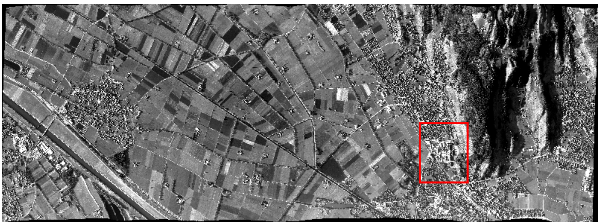
Figure 61 Panchromatic band from the strip imagery acquired with a forward look angle of 28° from the ADS40. Study area is highlighted in the red rectangle.
