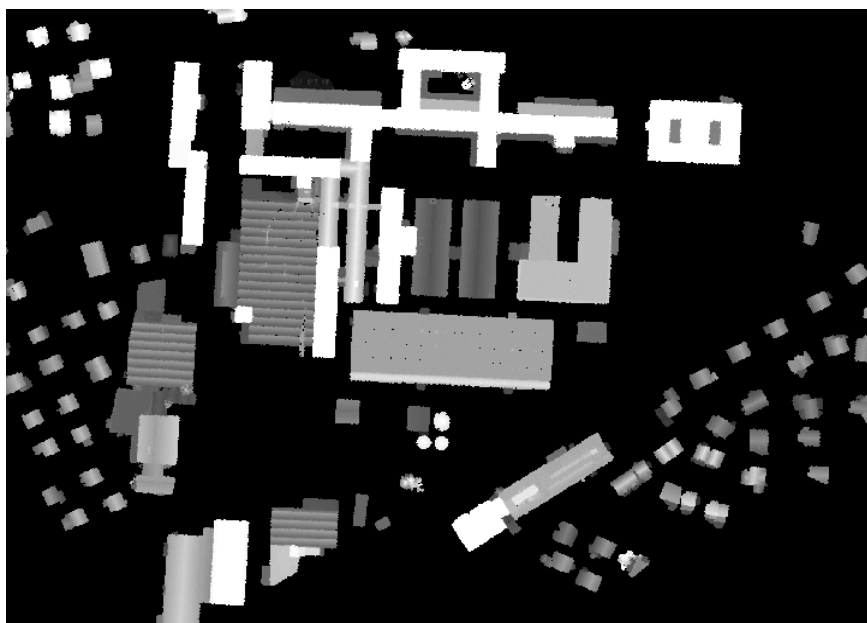
Figure 115 Digital Surface Model of the initial detected buildings and surrounding features in the background
