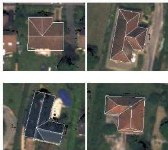
Figure 29 Reconstructed buildings projected on an orthophoto based on the method proposed by (Taillandier and Deriche, 2004).
