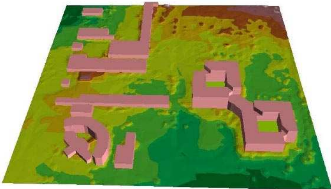
Figure 30 Final result from the reconstructed buildings overlaid on a DTM of the proposed method by NASA/ICREST Project report, (2001)
