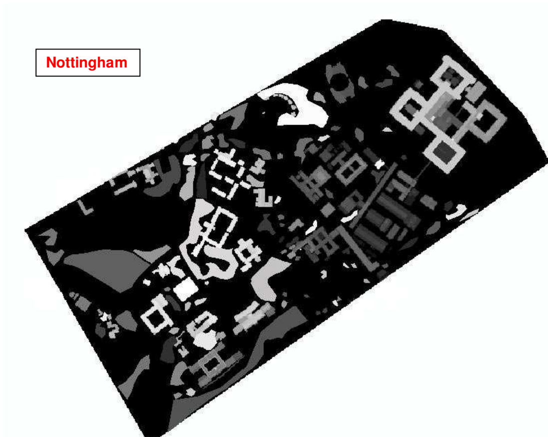
Figure 125 The merged image that contains both foreground and background objects after the implementation of size filtering and the components labelling algorithm. Different brightness values indicate different ID for each object
