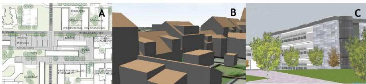
Figure 9 The three views of (Verbree et al., 1999) applicable at different stages in urban planning. a) PV, b) MV, and c) WV
