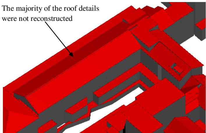
Building 12–single path LIDAR
