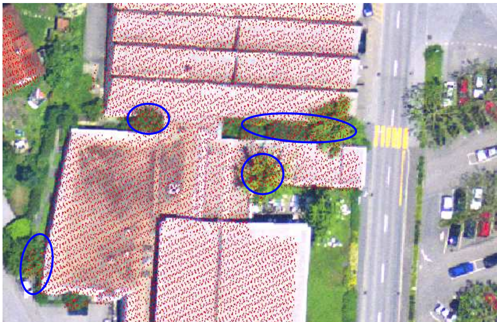
Figure 118 Incorrectly classified building points (highlighted in blue ellipses), superimposed on a rectified true colour composite
