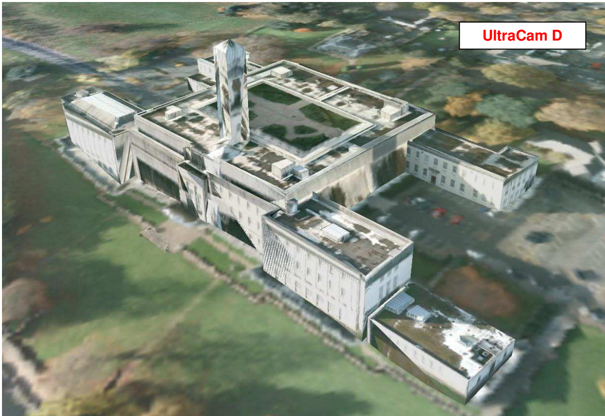
Figure 173 The automatically textured buildings models using the available Ultracam D airborne images with 80% overlap.
