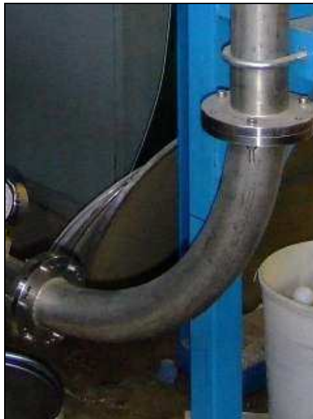
Figure 4.3: 220mm radii pipe ( R/D=4 )
