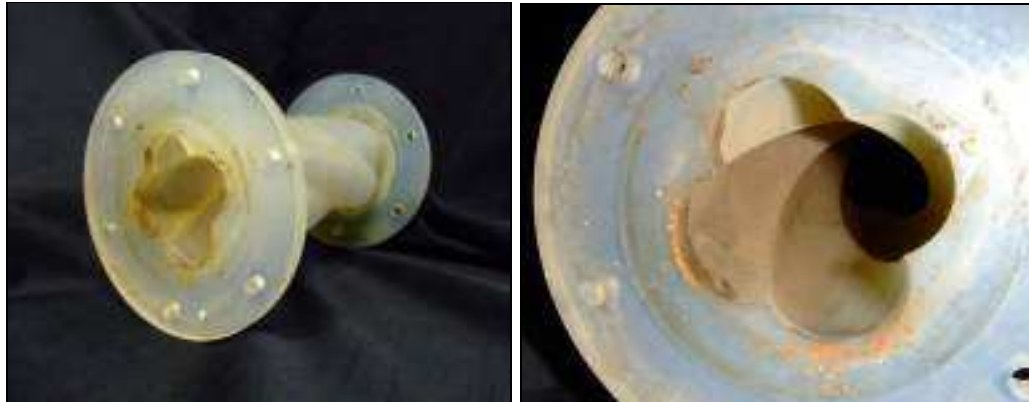
(a) Length = 20cm; diameter = 0.05m (b) View inside 4-lobe swirl pipe
