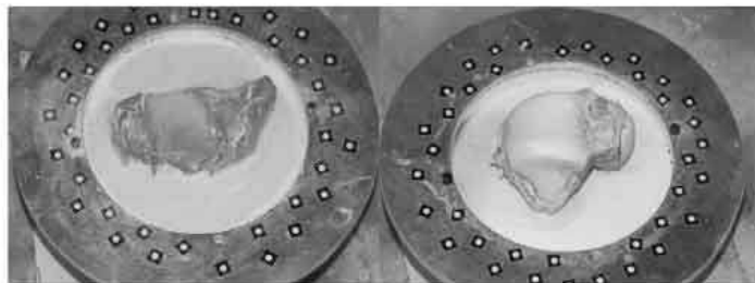
Fig. 1. A potted tibia–fibula complex and a talus specimen are shown in this picture. The articular surface of the talus has been prepared with a fine white powder to improve image contrast and optimise the performance of the ATOS system. Black and white photo targets are fixed to the flange on the potting cup.
