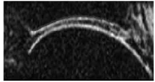
Fig. 6. Cartilage boundary tracking using directional gradient vector flow snake on the same image as in Fig. 1(a) and using the same initialization as in Fig. 1(b).
