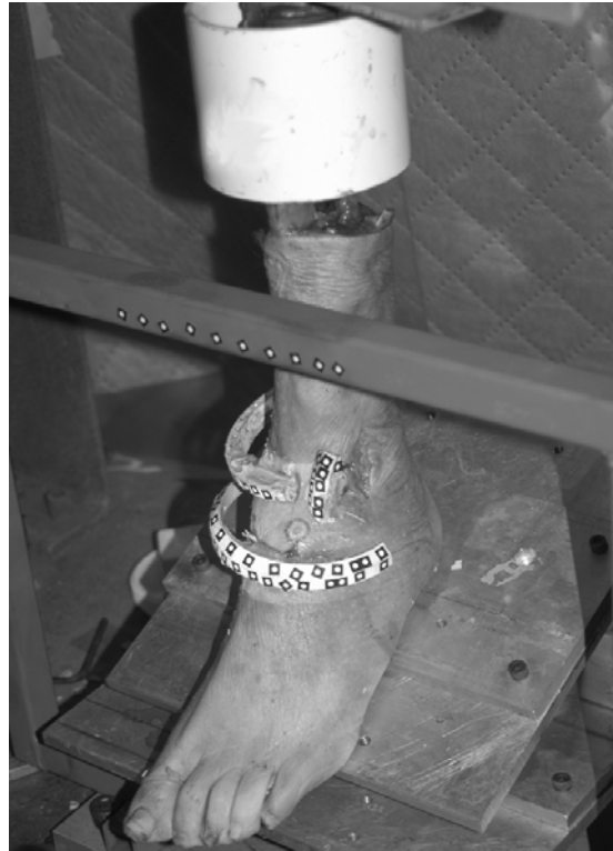
Figure 6.1 A lower leg specimen mounted in the test rig in 20° plantarflexion.
