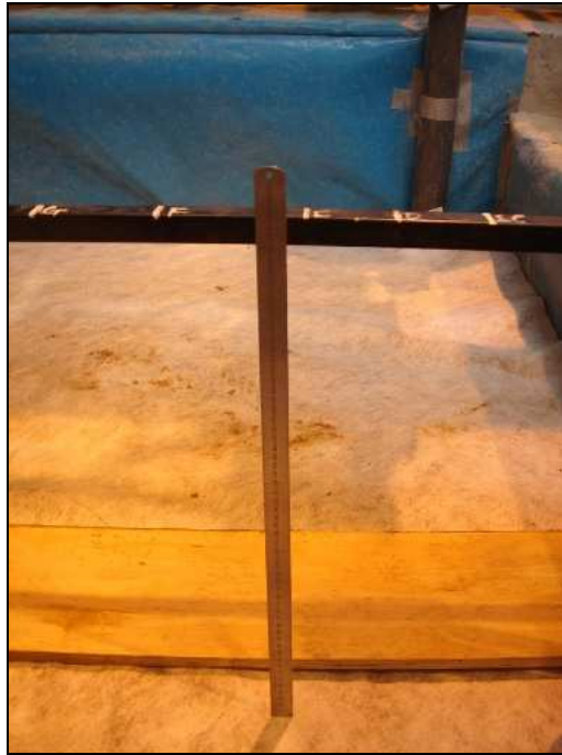
Figure 4.16. Measurement of subgrade profile
