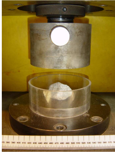
Figure 3.2. Configuration of a single particle crushing test
