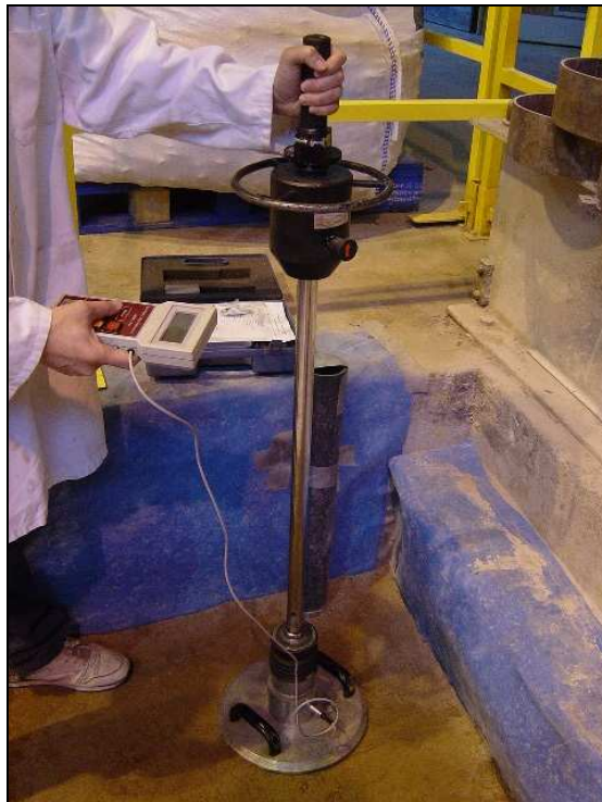
Figure 4.14. German Dynamic Plate measuring subgrade stiffness
