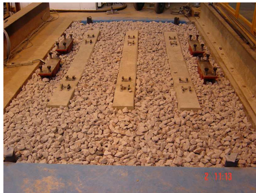
Figure 4.19. Sleeper arrangement in the RTF
