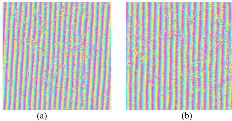
Figure 4. 6. Interferograms of the study area. (a) without flat earth correction and (b) with flat earth correction.
