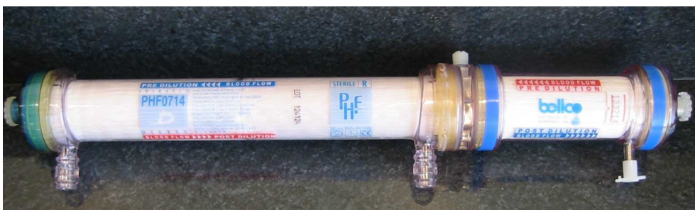
Figure 1-h. Double chamber dialyser used for PHF. The smaller chamber is the ultrafilter for the reinfusate, the larger chamber is the high flux haemodiafilter.
