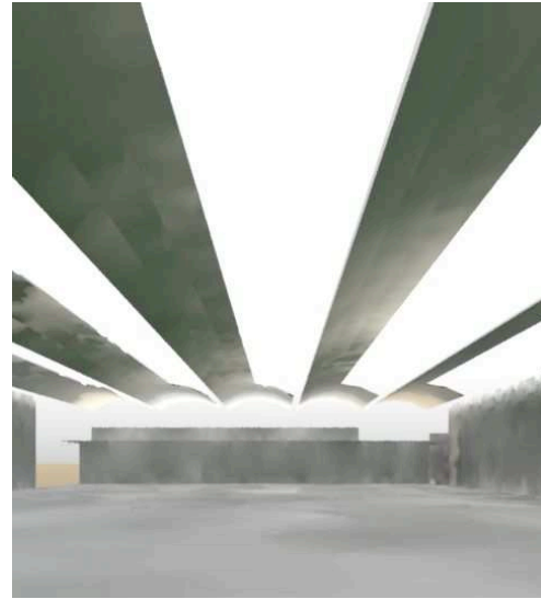
Fig. 6-25 Illuminance image of interior of the cricket school
