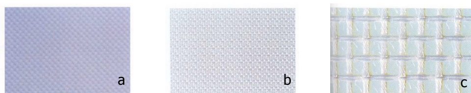
Fig. 2-15a PVC coated polyester; 2-15b Silicone-glass fibre; 2-15c PTFE glass.
