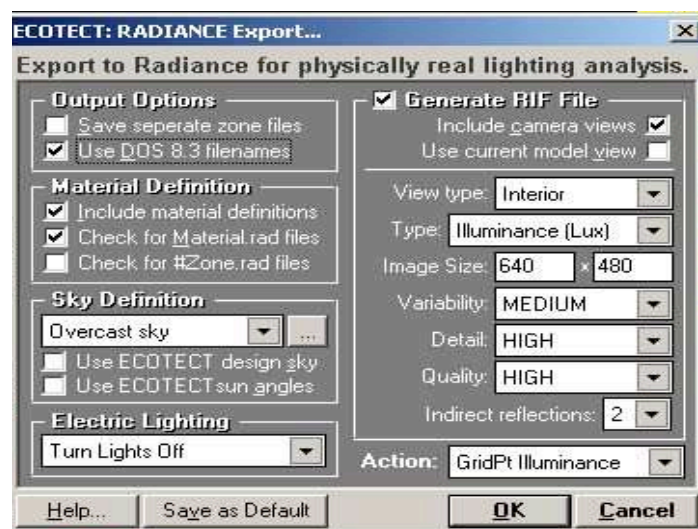
Fig. 6-17 Ecotect window for exporting files to Radiance
