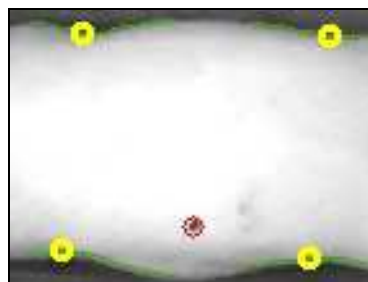
Figure 3.6 The four boundary kink detectors, and the predicted P2 point resting over a pre-marked P2 point for this test image.
