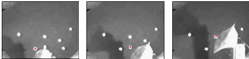
Figure 3.19 Example of a spot board testing of the positional accuracy of the robot in its final position. The spot board is placed at expected height of a pig and the user clicks on the white tape markers (20mm x 20mm) within the image analysis software. The robot should move such that the laser falls within the tape outline. The laser position has been highlighted for clarity. Mounted on the end of the robot arm are the observation camera and dust cover, and the laser.
