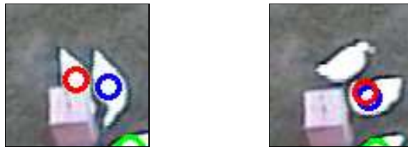
Figure 4.31 Left: two ducks come to feed. Right: approximately one second later, one of the targets has been ‘hijacked’ by one of the trackers. This problem occurs with multiple independent trackers where one target produces a higher quality measurement than the other.
