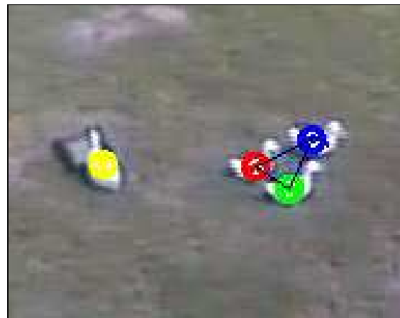
Figure 5.13 Example output frame from the MPS tracker. Three of the four targets’ movements are correlated above the threshold level, and hence three of the targets are grouped together as indicated by the lines – this is an example of automatic grouping as a consequence of the algorithm.
