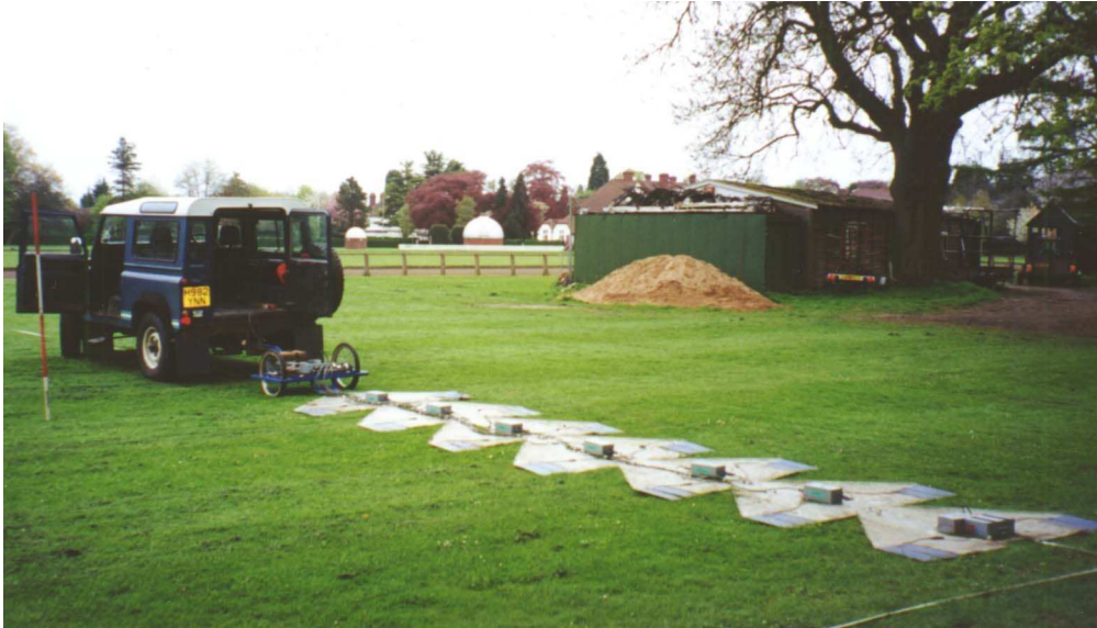
Figure 8.26: The CORIM™ system in field operation on the EIGG test site.
