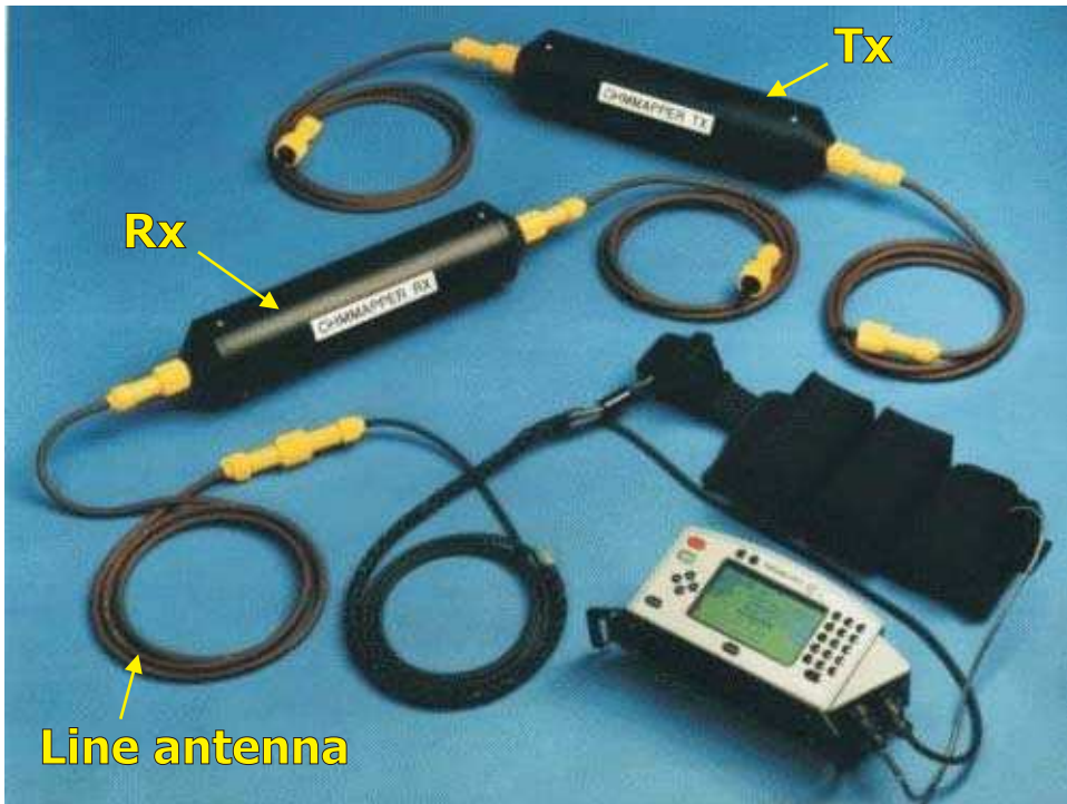
Figure 7.5: Components of the OhmMapper™ system. Photo: Geometrics Inc.
