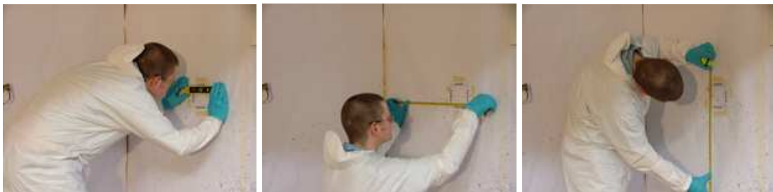
Figure 6-6- The levelling (left), and surface reference measurement of the horizontal (middle) and vertical (right) locations of the photographic scale in the sampled photographic recording of the two impact spatter patterns.
