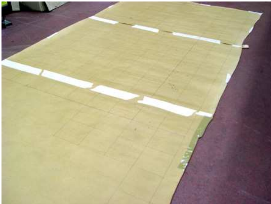
Figure 5-9 - The full target surface grid of pattern ES-C, expanded from the reference zone to cover the extremes of the impact spatter pattern.
