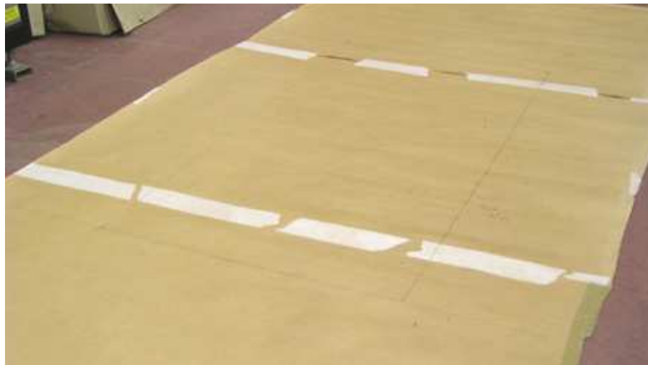
Figure 5-7 - The reference 0.5m by 1m zone marked on the target surface C during experimental impact spatter pattern production, with the vertical edges extended as the first stage in producing the target surface grid.
