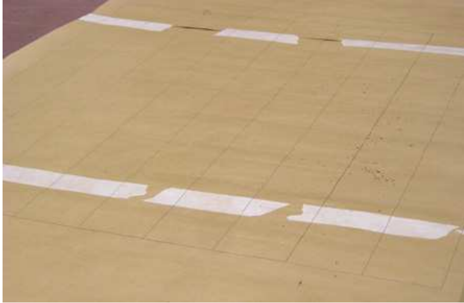
Figure 5-8 - Horizontal lines drawn every 10cm within the extended reference zone of pattern ES-C.
