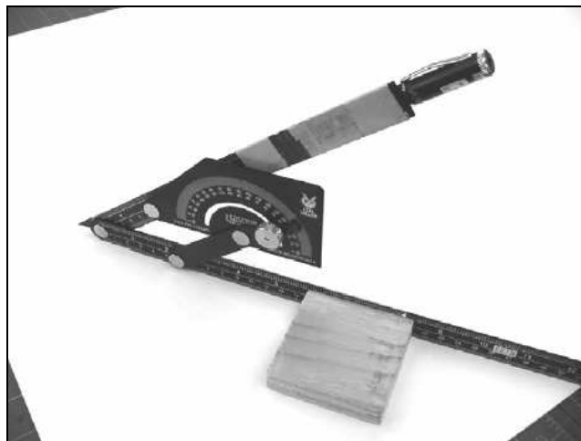
Figure 3-7 - A laser pointer developed for aiding the placement of strings as part of a 'stringing' site of impact estimation procedure (Mavin, 2002).
