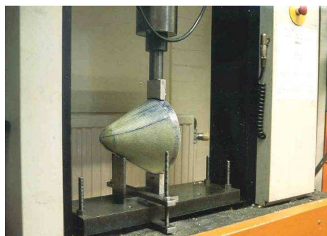
Figure 3.14 Jet engine nose cone mechanical test apparatus.
