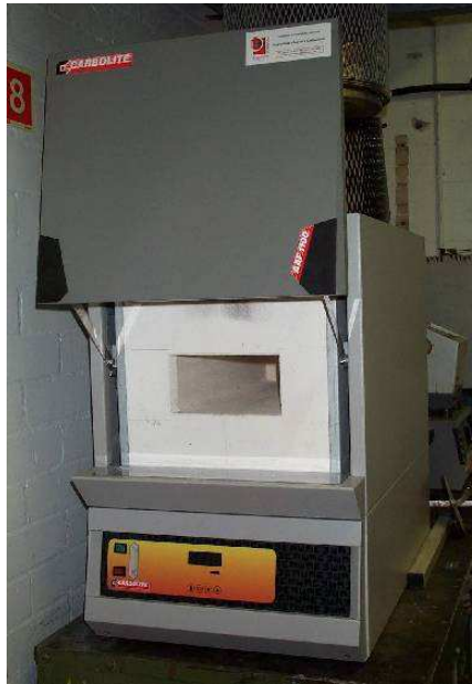
Figure 3.16 Carbolite AAF1100 electric muffle furnace used for fibre volume fraction measurement by ignition loss
