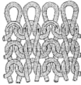
Figure 1.3 Schematic illustration of a weft-knitted textile (reproduced from [9])
