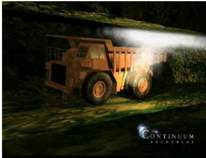
Figure 6-14: Haul truck on fire in decline
