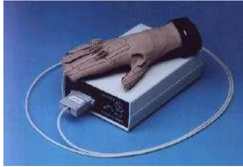
Figure 3.28: Data glove input device (after Virtex, 2000)
