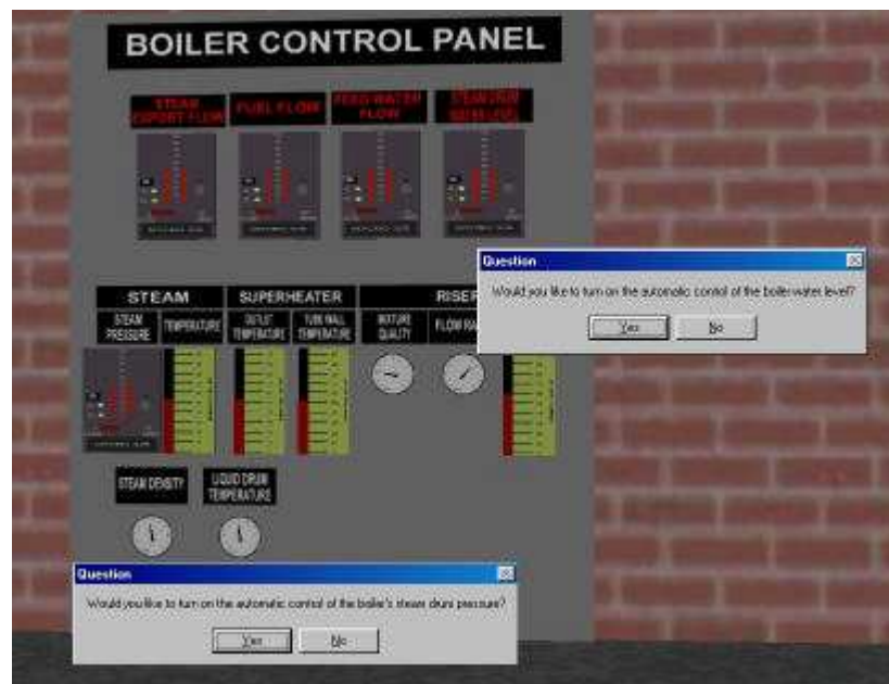
Figure 5.27: Boiler control panel. Prompt for automatic control
