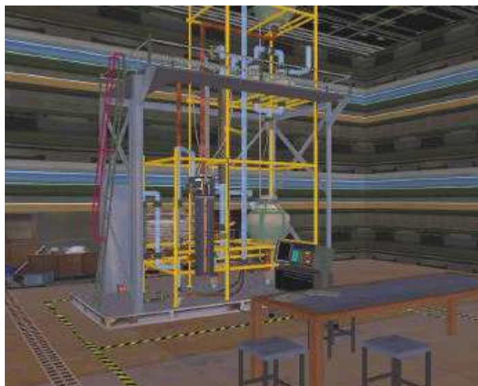
Figure 6.38: General view of the virtual reality absorption column experiment
