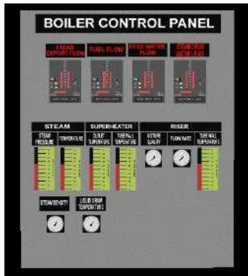
Figure 5.17: Perspective view of boiler's control panel
