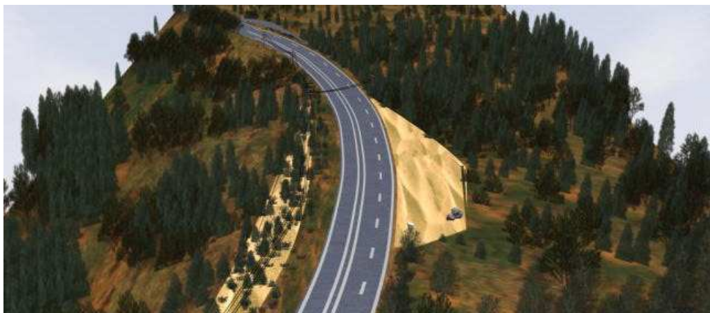
Figure 3.23: A view of the 3D computer model built, based on digital survey data and photographs (after Schofield et al , 2000).
