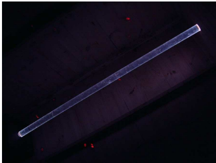
Fig. 4 - 10: Rod leakage in darkened chamber
