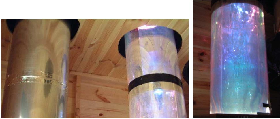
Fig. 7 - 11: Reference (95%) and 98% reflectance light pipes
