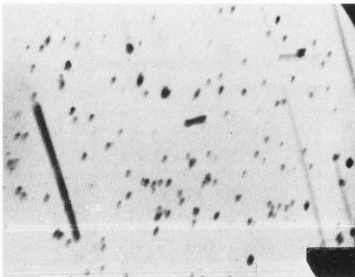
FIG.2 EBIC micrographs obtained from the same area of a GaP sample for different electron beam energies.
