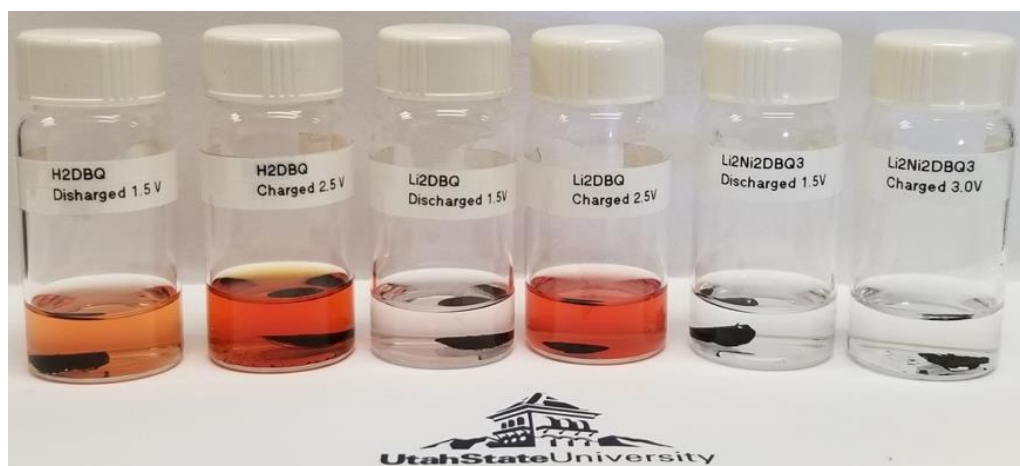
Figure 3-6. Photography of charged and discharged electrodes in 1.0 M LiTFSI in 1:1 V:V DME:DOL of \text{H}_2\text{DBQ} , \text{Li}_2\text{DBQ} , and \text{Li}_2\text{Ni}_2\text{DBQ}_3 (from left to right).
