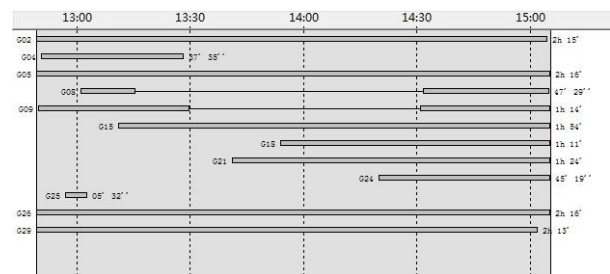
Figure 5: Satellites' visible time during field test
