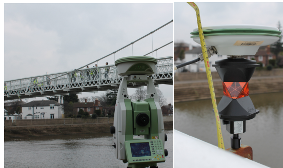
Fig. 2: The RTS with the GPS station for recording in GPS time (left) and the GPS antenna with the reflector mounted on the handrail at the midspan of the bridge (right).
