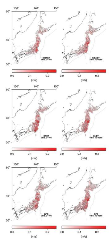
**Figure 6b**: Maximum ground velocity maps for KiK-net (top), K-NET (middle), and GPS (bottom) for the two period bands (3-10s and 10-100s).
