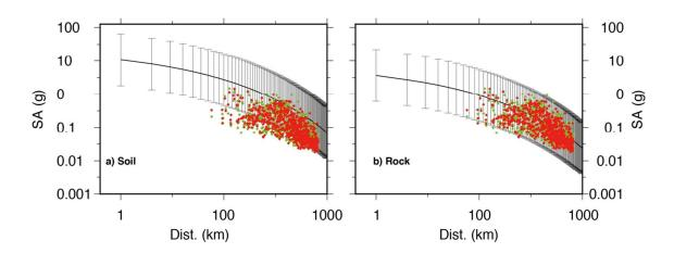
**Figure 9**: Spectral acceleration (SA) at 3s from GMPE (black line) of soft soil (a) and bedrock (b) conditions (Zhao et al., 2006) compared to the SA computed from GPS (red dots) and to the SA computed from the strong-motion records (green dots). The error bars indicate the  $1\sigma$  uncertainty zone of the GMPE.
