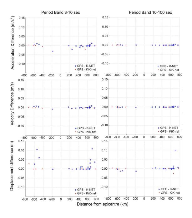
**Figure A1**: The differences of the GPS and strong-motion MGA (top), MGV (middle) and MGD (bottom) values for each very closely located sites versus the distance from the epicentre. The positive and negative distances correspond to the position of the sites northward and southward from the epicentre.
