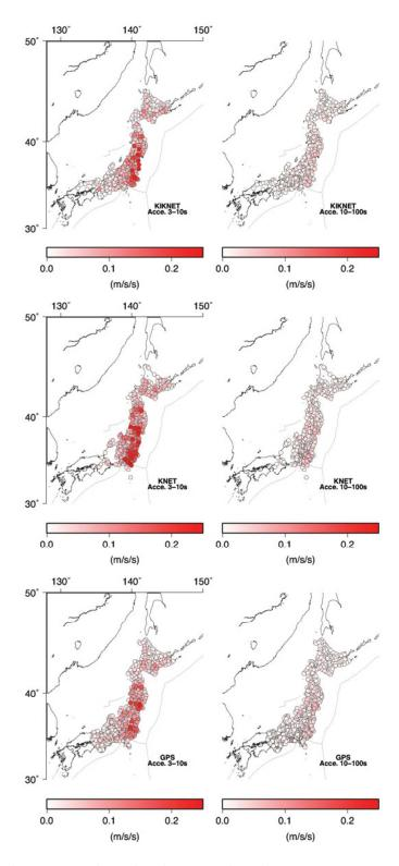
**Figure 6a**: Maximum ground acceleration maps for KiK-net (top), K-NET (middle), and GPS (bottom) for the two period bands (3-10s and 10-100s).
