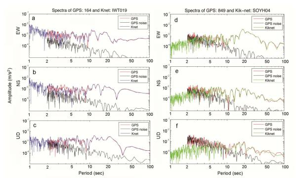
**Figure 4**: Spectra of derived acceleration time series using K-NET, KiK-net and GPS data for two sites: (a-c) close (179km) and (d-f) far (771km) from the epicentre. The solid black line corresponds to the spectra of the GPS acceleration time series before the occurrence of the earthquake indicating the noise level.
