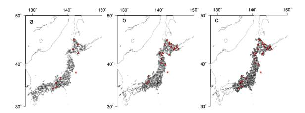
**Figure 3**: KiK-net (a), K-NET (b) and GEONET GPS (c) sites used in this study. The very closely located sites of GPS and strong-motion networks are indicated with red triangles. The red star indicates the epicentre of the Tohoku-Oki earthquake in 2011.
