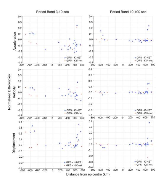
**Figure 8**: Normalised differences of GPS and strong-motion MGA (top), MGV (middle) and MGD (bottom) at the very closely located sites. The positive and negative distances correspond to the position of the sites northward and southward from the epicentre.
