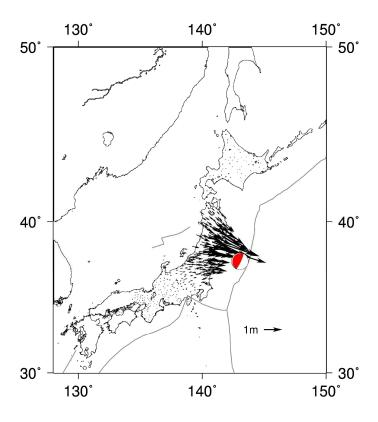
**Figure 2**: Precise Point Positioning (PPP) coseismic horizontal displacement field for the Tohoku-Oki event measured by the GEONET GPS network at  $t = T_0 + 300s$ .
