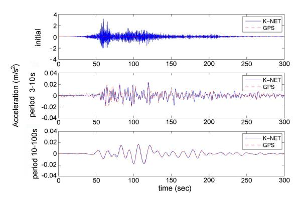
**Figure 5**: The initial acceleration time series of the very closely located sites of K-NET IWT019 (blue solid line) and GPS 0164 (dashed red line) and the derived time series after filtering for the 3-10s and 10-100s period bands. The time corresponds to seconds since the earthquake occurrence.
