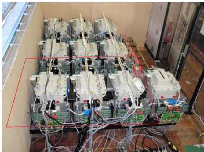
Fig. 9. UNIFLEX-PM power converter in place for low voltage testing: (a) complete 12-cell setup for 3-phase 3-port operation, (b) highlighted cells used for single-phase 2-port operation.
