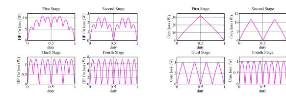
(a) High frequency Copper loss in the magnetic components
