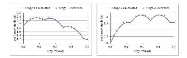
(a) Peak-to-peak ripple in stage-1 channel current
