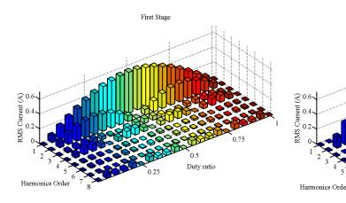
(a) Harmonics components in the stage-1 current
