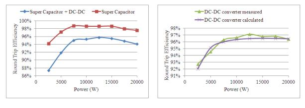
(b) Measured round-trip efficiency of super-capacitor and super-capacitor+dc-dc converter
