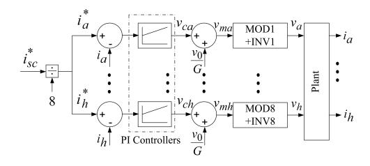
(a) Block diagram of the current controller
