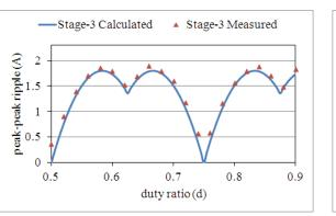
(c) Peak-to-peak ripple in stage-3 channel current
