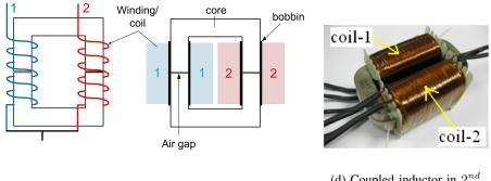
(c) Physical construction of the coupled inductors
