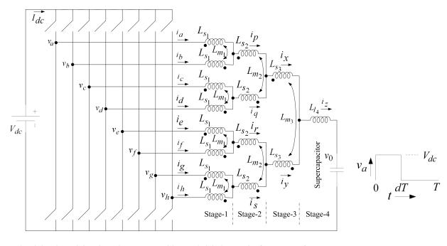
(d) Eight channel interleaved converter with coupled inductors in four stages for supercapacitor interface (e) Voltage  $v_a$  with time
