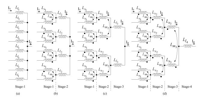
Fig. 2. 4 topologies under comparison: (a) 1-stage topology, (b) 2-stage topology, (c) 3-stage topology, (d) 4-stage topology
