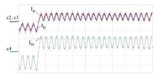
(a) With  $kp = 75m\Omega$ ; c2 and c3:  $I_a$  and  $I_b$  (5A/div), c4: Isc (20A/div), time: 500  $\mu$ sec/div
