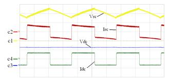
(a) Super capacitor charge discharge cycling at 20kW, c1: Vsc (100V/div), c2: Isc (100A/div), c3: Vdc (200V/div), c4: Idc (75A/div), time: 20 s/div
