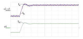
(d) Large step change with  $kp = 25m\Omega$ ; c2 and c3:  $I_a$ and  $I_b$  (5A/div), c4: Isc (50A/div), time: 200  $\mu$ sec/div
