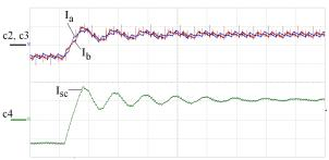
(b) With  $kp = 50m\Omega$ ; c2 and c3:  $I_a$  and  $I_b$  (5A/div), c4: Isc (20A/div), time: 200  $\mu$ sec/div
