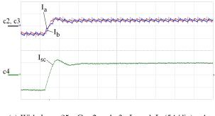
(c) With  $kp = 25m\Omega$ ; c2 and c3:  $I_a$  and  $I_b$  (5A/div), c4: Isc (20A/div), time: 200  $\mu$ sec/div
