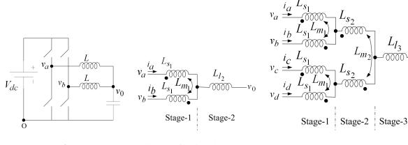
(a) Topology of a two channel DC-DC converter in parallel
