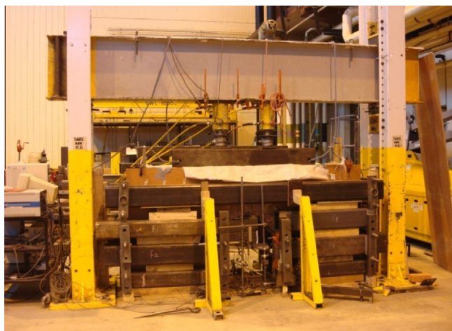
Fig. 3. Loading system installation for uniform load.
