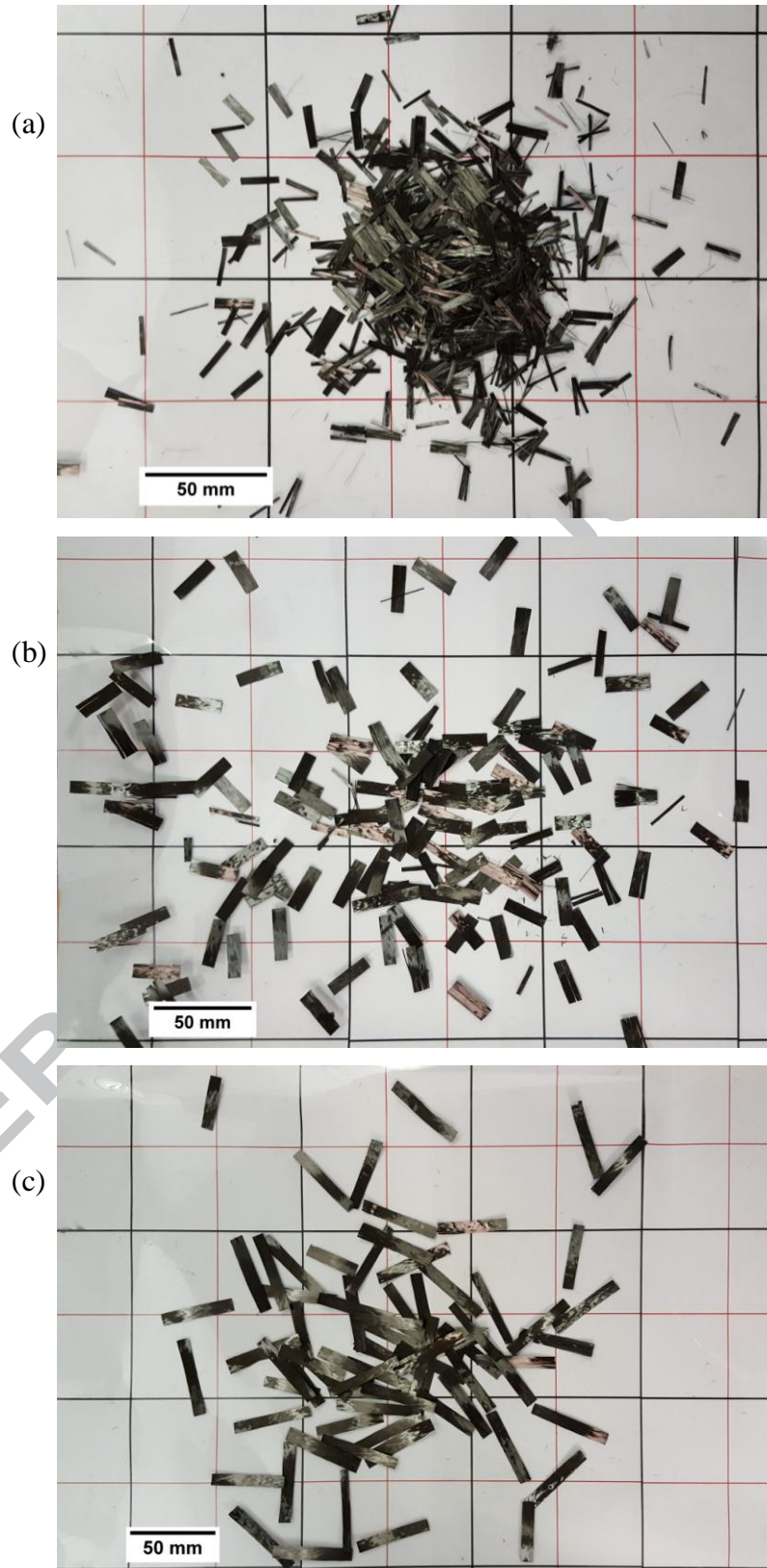
Figure 11: Dry deposition of (a) 15mm (b) 25mm and (c) 50mm fibre lengths, showing increasing levels of tow fragmentation for shorter bundle lengths.
