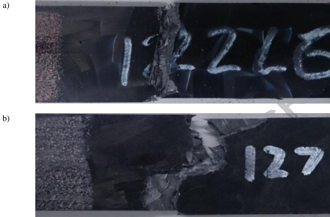
Figure 5: Typical failure mechanisms experienced during tensile failure of longitudinal specimens of (a) 100% mould coverage DFC, (b) 50% mould coverage DFC
