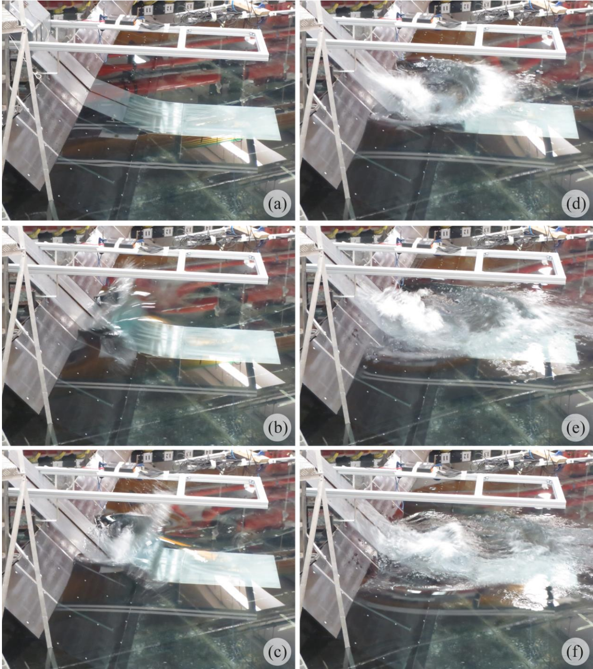
Fig. 6. Series of images of slide impact and tsunami generation in 3D for a test with F = 1.15 , S = 0.25 and M = 0.25 ; the time interval from (b) onwards is 0.2 s.
