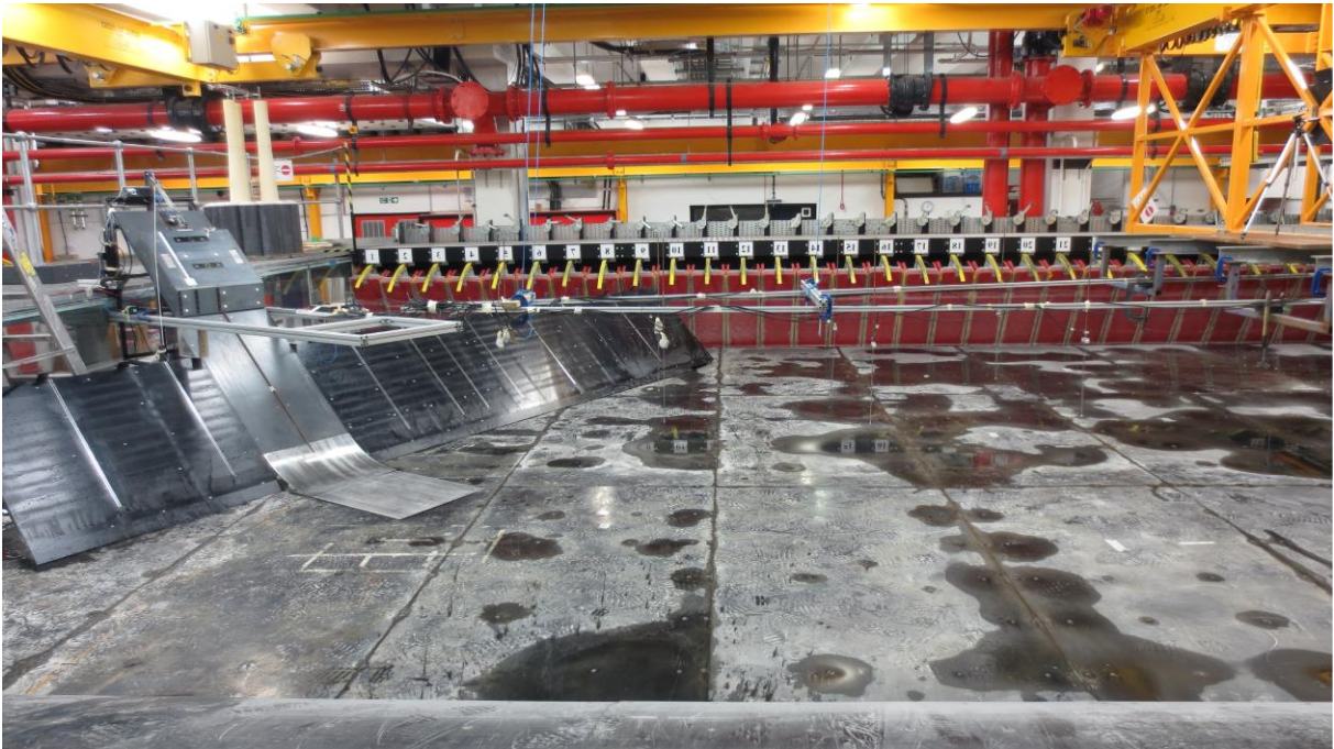
Fig. 1. Wave basin set-up in position 2 showing on the left: medium slide on ramp, circular transition and steel plate on ramp toe and side-walls with run-up gauges; centre: first wave probes at r/h = 3.0, 5.0, 7.5 and 10.0 for \gamma = 30^\circ and 45^\circ and h = 0.480 m; right: bridge supporting the beams hosting the wave probes and tripod for video recordings; note that the set-up was relocated for the measurements at \gamma = 0^\circ, 15^\circ (position 1) and at 58^\circ, 73^\circ and 90^\circ (position 3) and the side walls were extended in position 3.
